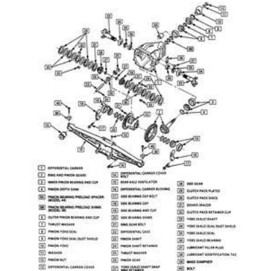
Fig. 2: Exploded view of the rear axle components — 1996 vehicle shown, others similar
