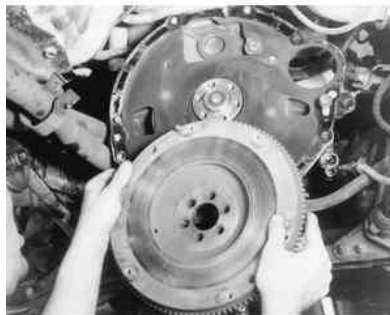
Fig. 6: . . . then remove the flywheel from the crankshaft in order to replace it or have it machined
