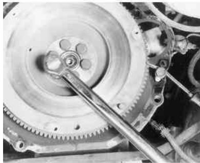
Fig. 5: If necessary, lock the flywheel in place and remove the retaining bolts . . .
