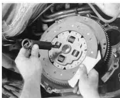
Fig. 7: Install a clutch alignment arbor, to align the clutch assembly during installation
