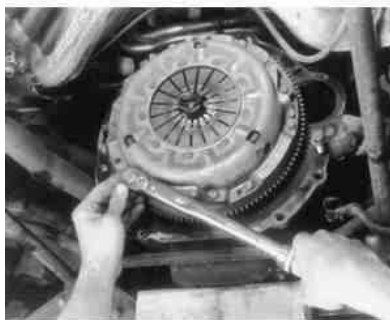
Fig. 9: Be sure to use a torque wrench to tighten all bolts
