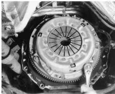
Fig. 2: Loosen and remove the clutch and pressure plate bolts evenly, a little at a time . . .
