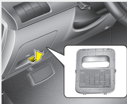
Inner fuse panel
