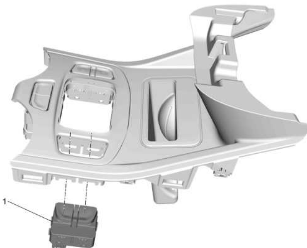
Fig. 18: Front Seat Heater Switch (Terrain). Courtesy of GENERAL MOTORS COMPANY
