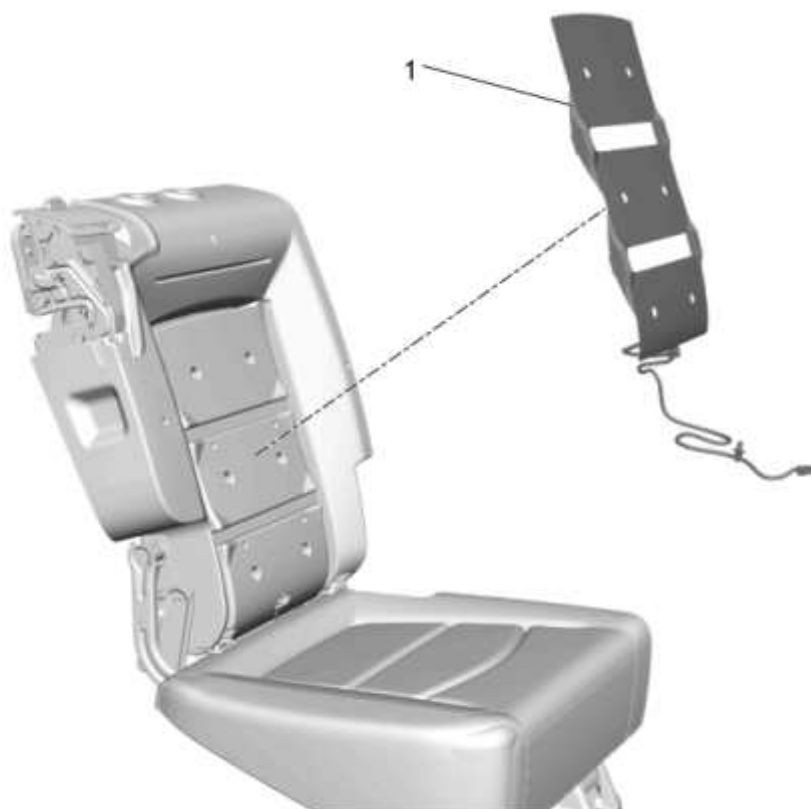
Fig. 24: Rear Seat Back Cushion Heater Courtesy of GENERAL MOTORS COMPANY
