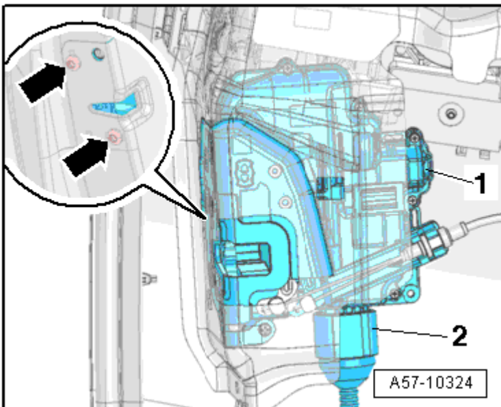
Fig. 32: Identifying Door Lock, Removal Courtesy of AUDI OF AMERICA, LLC
