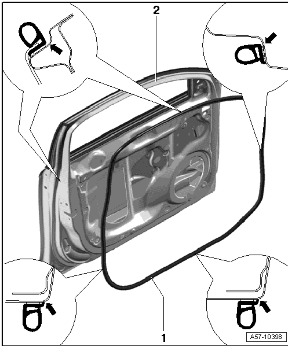
Fig. 41: Marking Distances And Then Press The Seal On Courtesy of AUDI OF AMERICA, LLC
