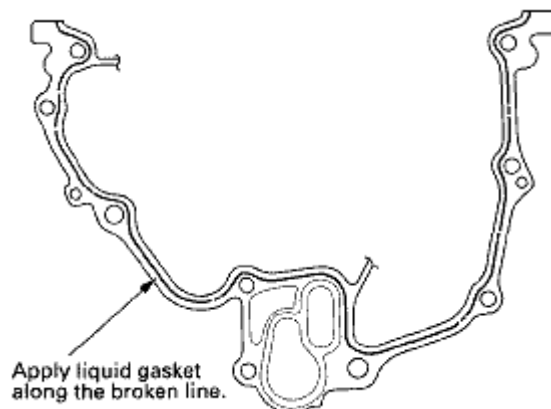
Fig. 20: Identifying Liquid Gasket Applying Area
