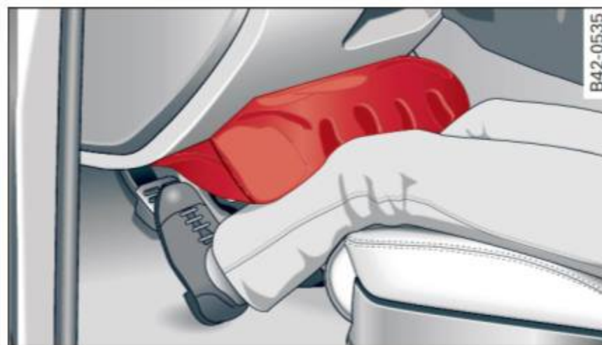
Fig. 120 Inflated airbags protecting in a frontal collision
