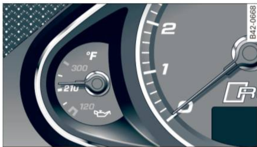
Fig. 138 Instrument cluster: Engine oil temperature display
