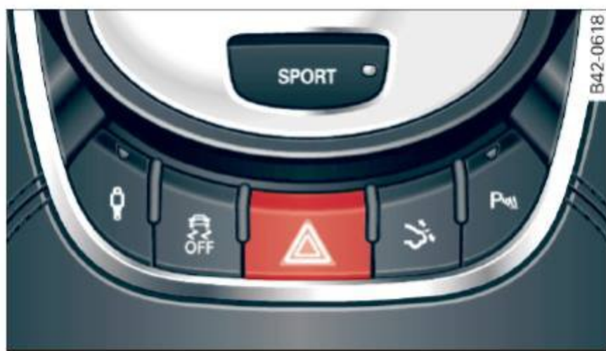
Fig. 57 Center console: emergency flasher switch
