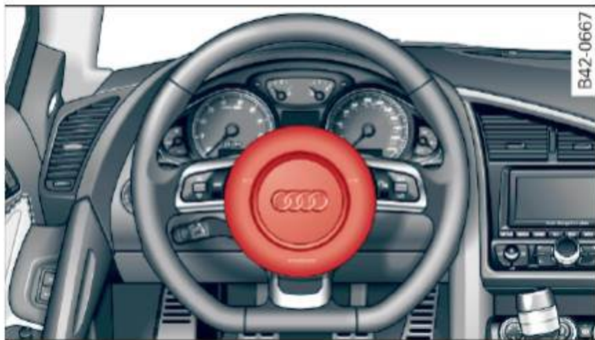
Fig. 115 Location of driver airbag: in steering wheel
