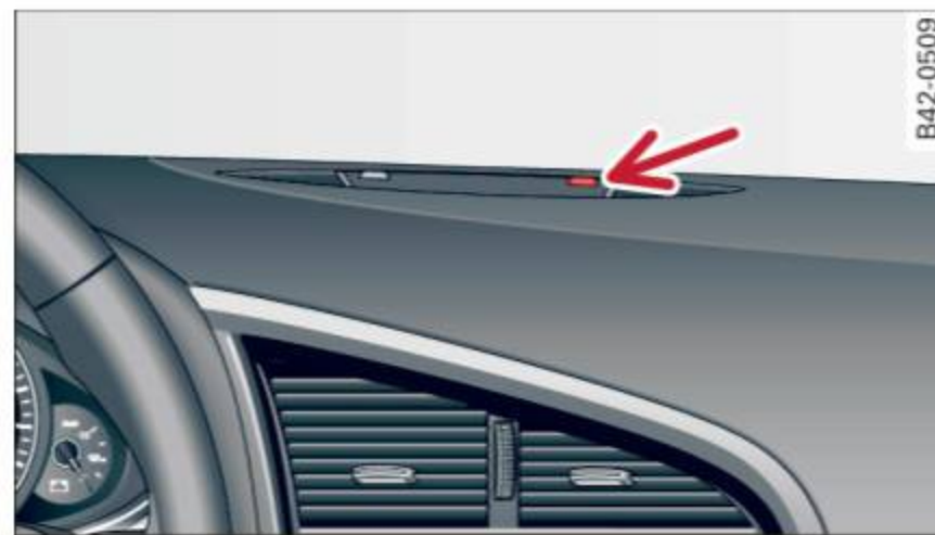
Fig. 30 Diode position in the instrument panel
