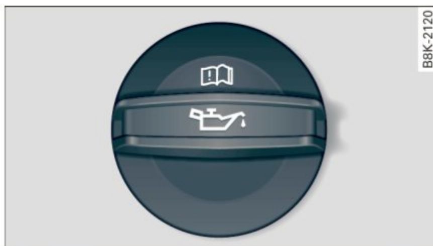
Fig. 141 Engine compartment: cover on the engine oil filler neck
