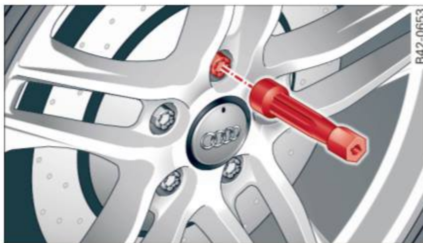
Fig. 159 Wheel change: using the screwdriver handle (with the blade removed) to turn the bolts
