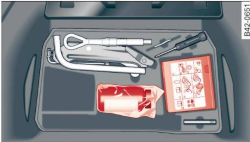
Fig. 153 Tire Mobility System under luggage compartment floor
