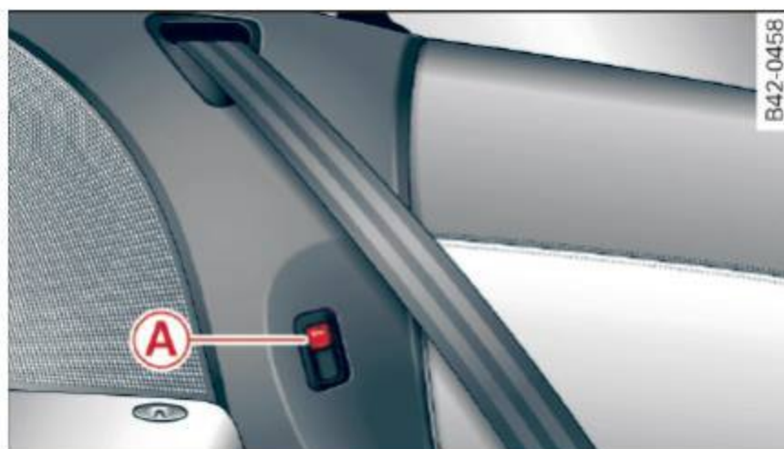
Fig. 132 Driver's side: releasing the engine compartment lid
