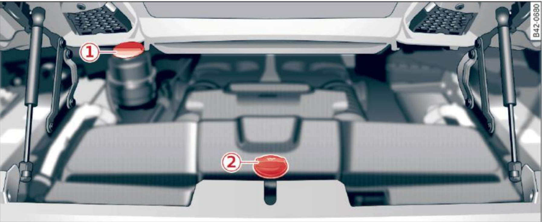
Fig. 135 Typical layout for containers, engine oil dipstick and engine oil filler cap (S tronic)
