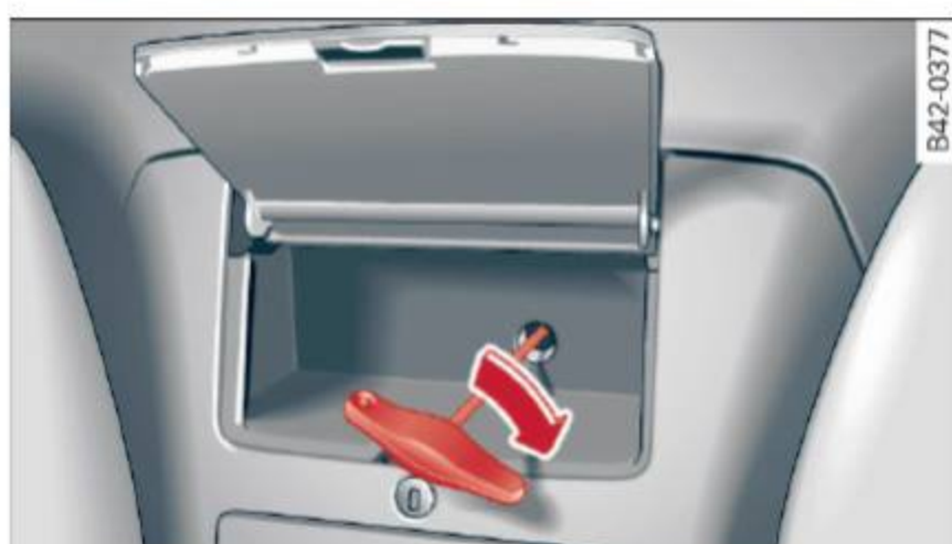
Fig. 41 Upper storage compartment: using the Allen wrench as a crank to lower the rear window
