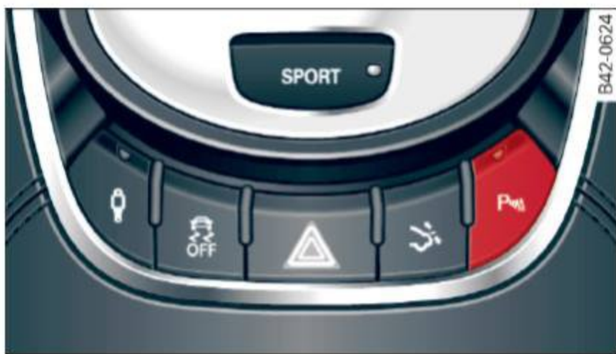
Fig. 93 Section of the center console: Park assist switch
