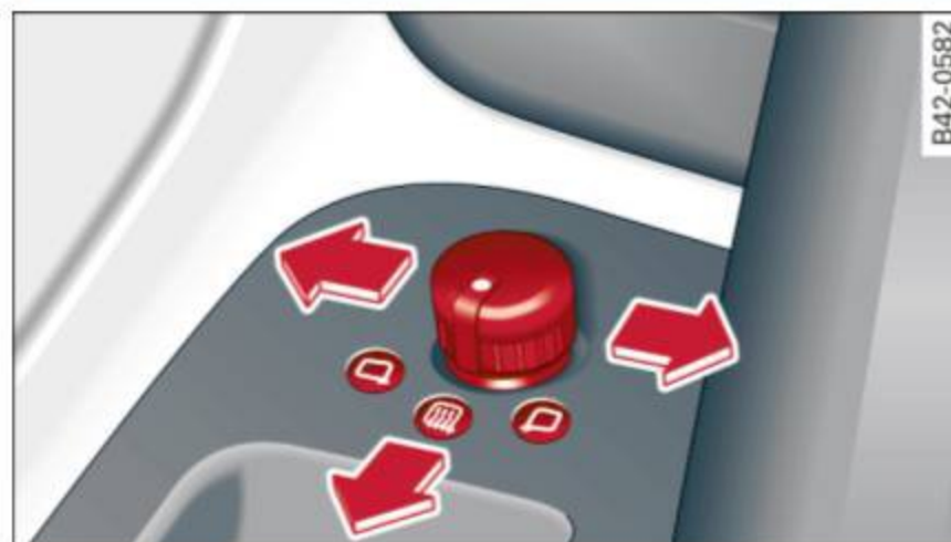
Fig. 60 Forward section of driver's armrest: power mirror controls
