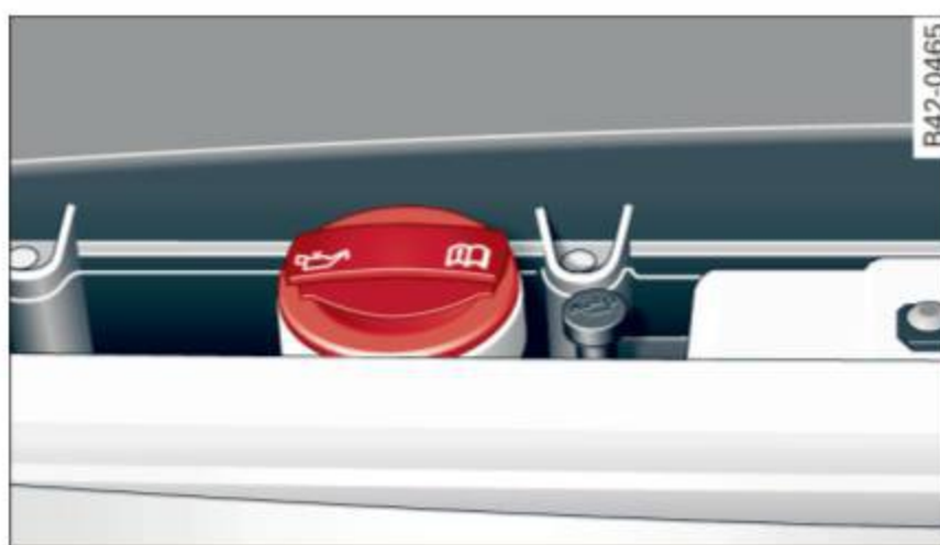
Fig. 140 Engine compartment: Oil filler cap location
