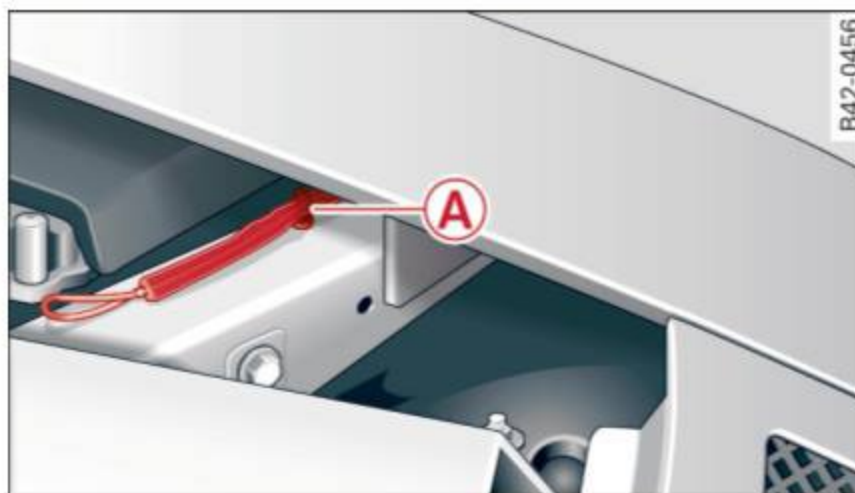
Fig. 130 Engine compartment: loosening the fuel filler flap cable
