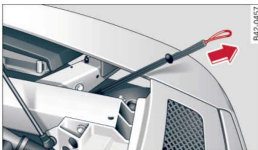
Fig. 131 Engine compartment: releasing the fuel filler flap using the emergency release
