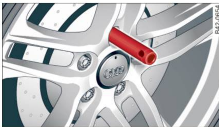
Fig. 160 Wheel change: alignment pin inside the top hole
