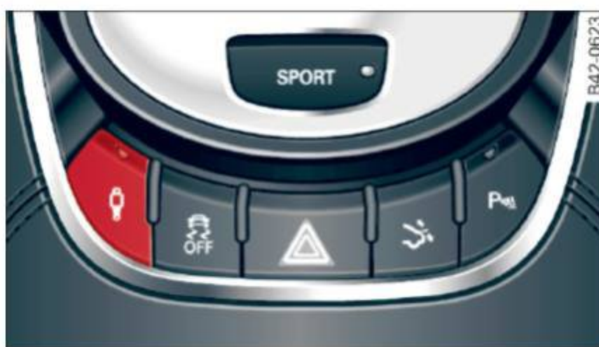
Fig. 82 Center console: Switch for Audi magnetic ride
