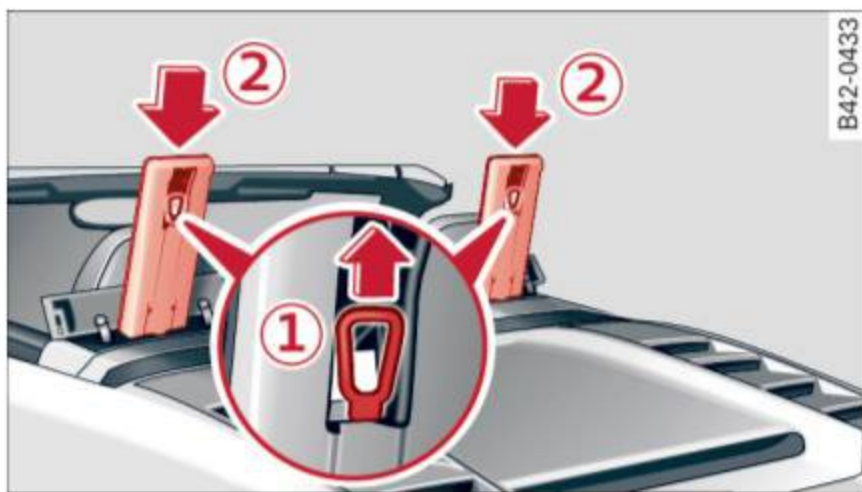
Fig. 104 Deployed rollbar with release loop
