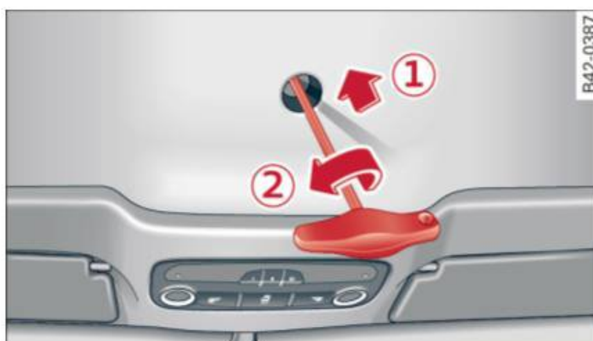
Fig. 51 Inner side of the convertible top: positioning the Allen wrench
