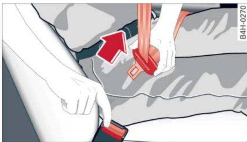
Fig. 114 Releasing the tongue from the buckle
