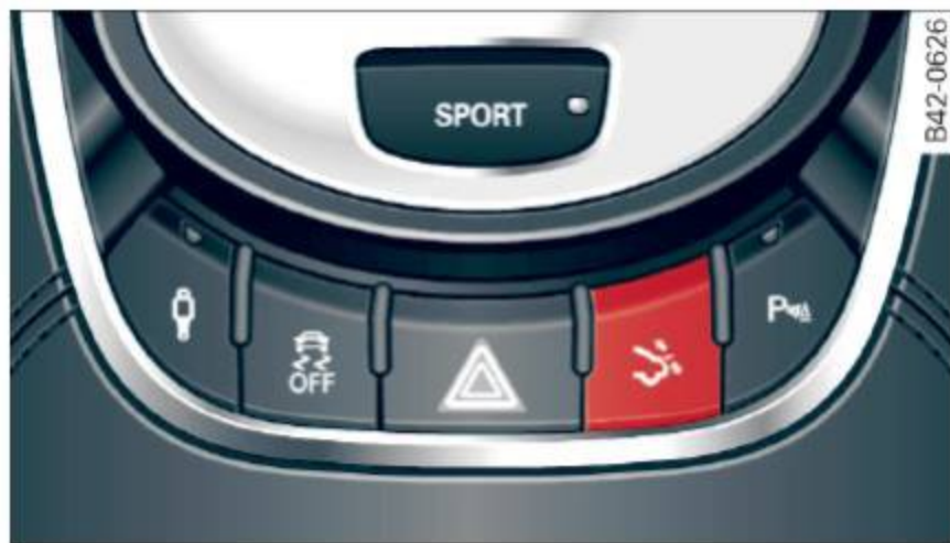
Fig. 127 Switch for rear spoiler
