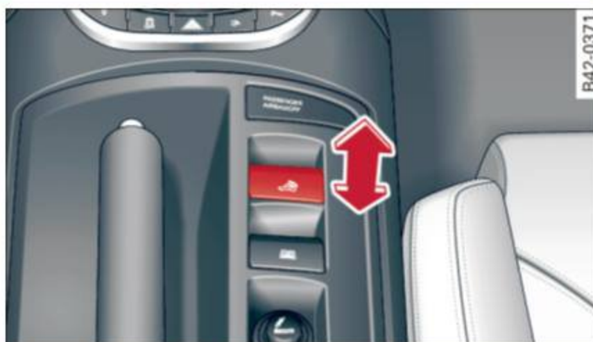
Fig. 35 Center console: convertible top switch
