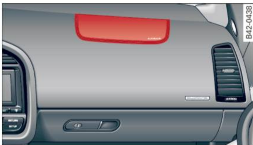
Fig. 116 Location of front passenger's airbag: in the instrument panel
