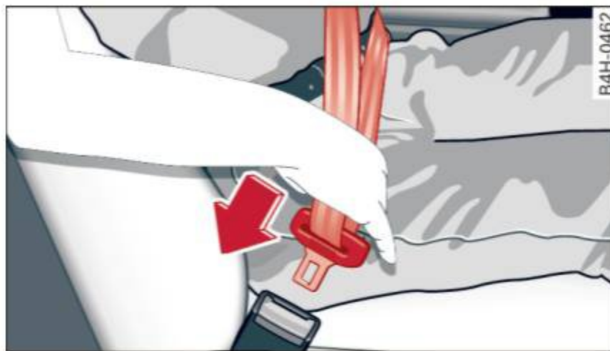
Fig. 111 Belt buckle and tongue on the driver's seat
