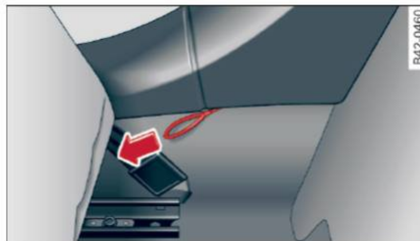
Fig. 133 Front passenger footwell: emergency release loop
