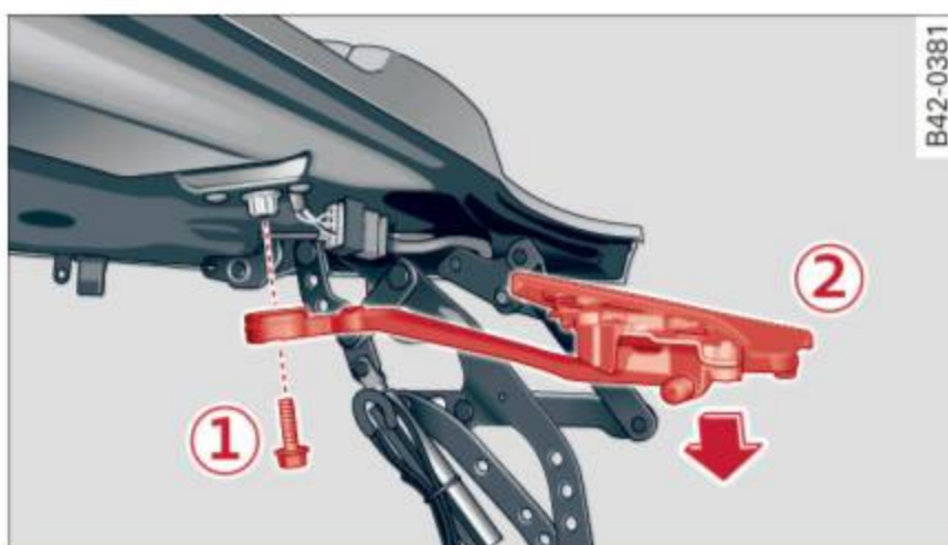
Fig. 45 Convertible top storage bay lid: removing the cover
