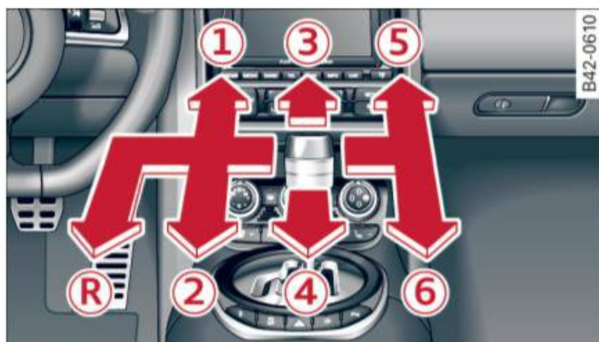
Fig. 83 Gearshift pattern: 6-speed manual transmission
