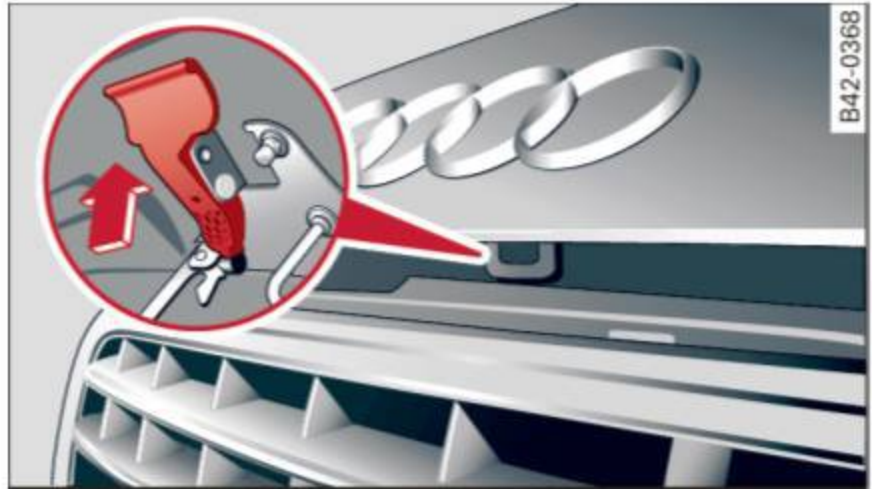
Fig. 28 Release lever under the front lid
