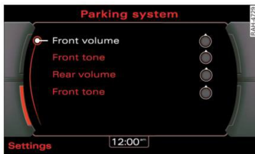
Fig. 99 Navigation system display: adjusting the parking system
