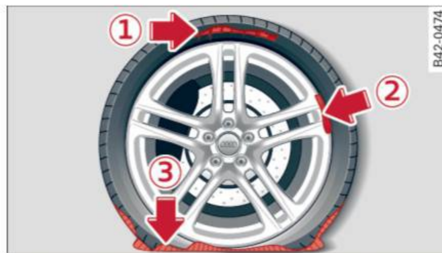
Fig. 152 Tire damage for which the Tire Mobility System is not suited
