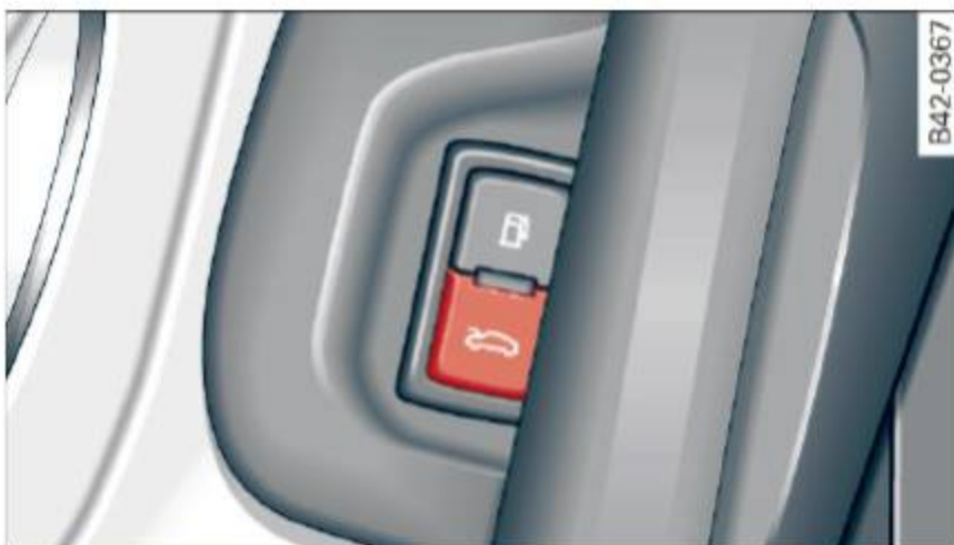
Fig. 27 Drivers door: remote front lid release
