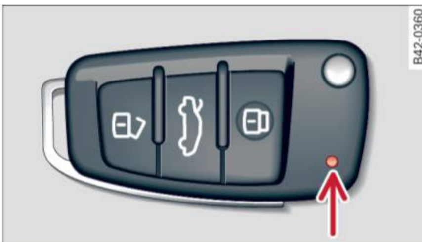
Fig. 21 Remote master key: Indicator light
