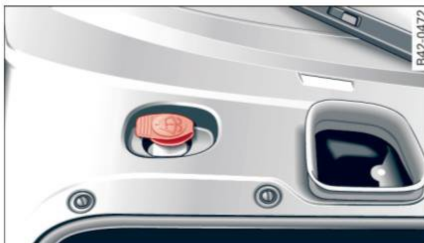
Fig. 146 Luggage compartment: Windshield washer fluid reservoir
