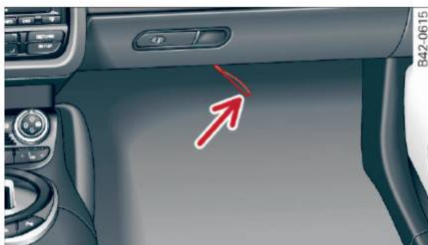
Fig. 29 Section: Emergency release
