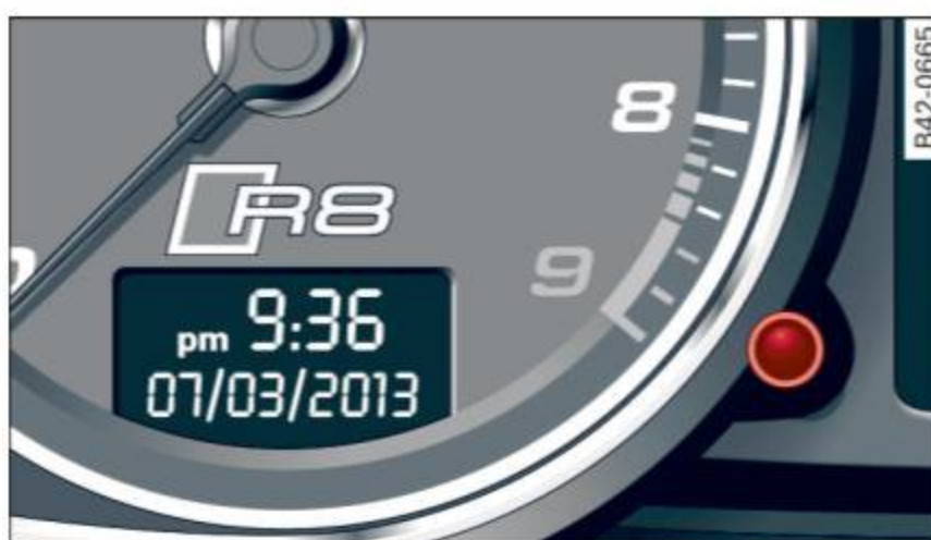
Fig. 79 Section of instrument cluster: Set/Check button
