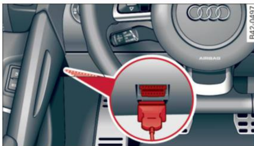
Fig. 19 Location of Data Link Connector (DLC)
