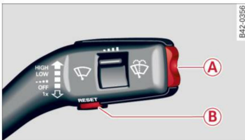
Fig. 12 Wiper lever: Controls for the menu display
