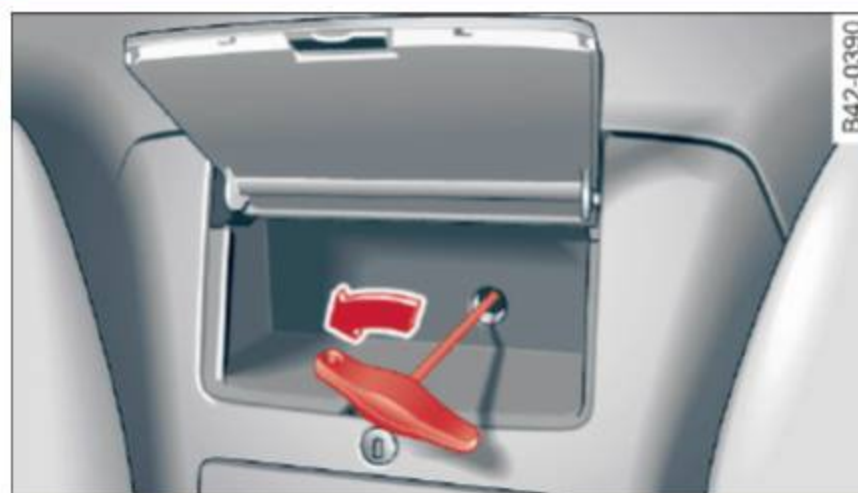
Fig. 54 Upper storage compartment between the seat backrests: extending the rear window
