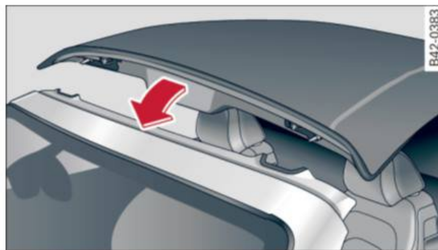
Fig. 47 Windshield frame: pressing the convertible top forward
