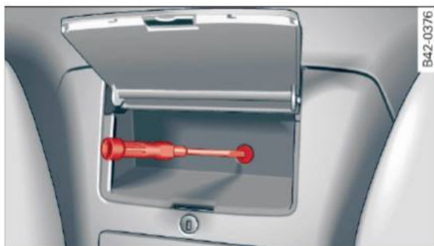
Fig. 40 Upper storage compartment: removing the cover
