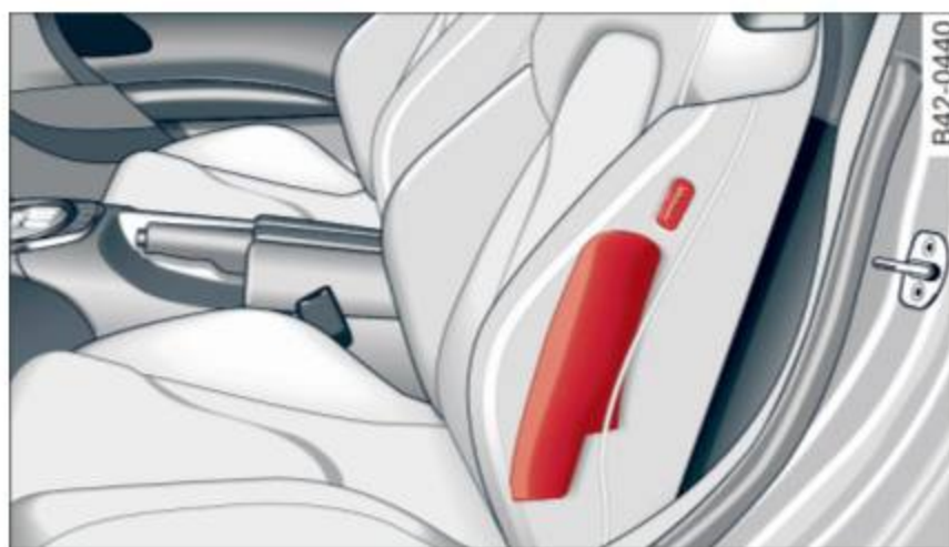
Fig. 121 Side airbag location in the driver's seat
