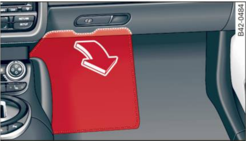
Fig. 164 Passenger's side wheel well: Foot rest with fuse arrangement
