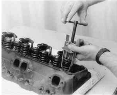
Fig. 1: When removing an OHV valve spring, use a compressor tool to relieve the tension from the retainer
