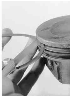
Fig. 5: Checking the piston ring-to-ring groove side clearance using the ring and a feeler gauge
