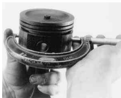
Fig. 2: Measure the piston's outer diameter, perpendicular to the wrist pin, with a micrometer
