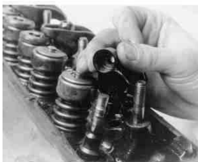
Fig. 5: Removing an umbrella/positive type seal
