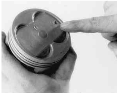
Fig. 2: Most pistons are marked to indicate positioning in the engine (usually a mark means the side facing the front)
