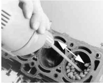
Fig. 1: Use a ball type cylinder hone to remove any glaze and provide a new surface for seating the piston rings
