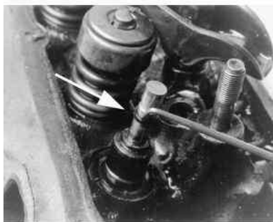
Fig. 5: Removing an umbrella/positive type seal
