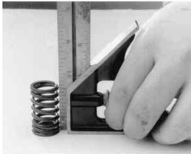
Fig. 4: Check the valve spring for squareness on a flat surface; a carpenter's square can be used
