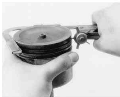
Fig. 3: Clean the piston ring grooves using a ring groove cleaner tool, or . . .
