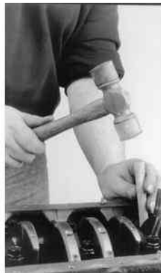
Fig. 2: Carefully tap the piston out of the bore using a wooden dowel
