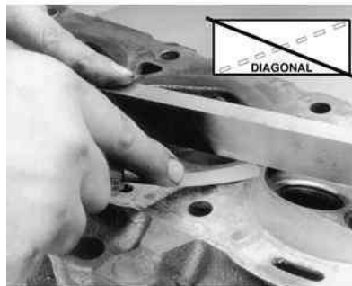
Fig. 7: Checks should also be made along both diagonals of the head surface
