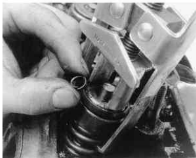
Fig. 3: Be careful not to lose the small valve locks (keepers)
