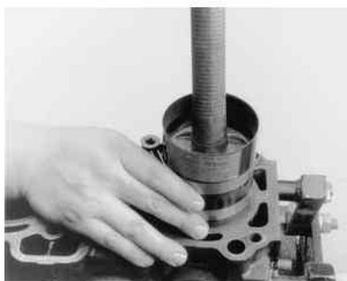
Fig. 8: Install the piston and rod assembly into the block using a ring compressor and the handle of a hammer
