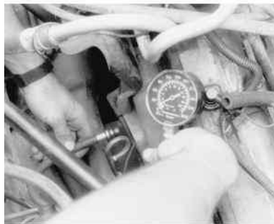
Fig. 1: A screw-in type compression gauge is more accurate and easier to use without an assistant
