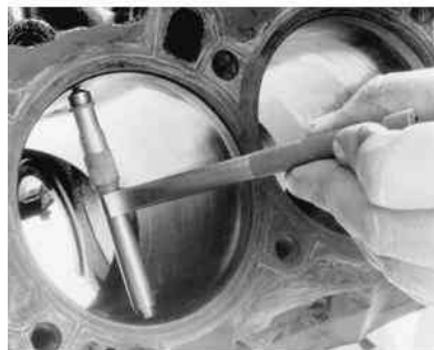
Fig. 1: Use a telescoping gauge to measure the cylinder bore diameter — take several readings within the same bore
