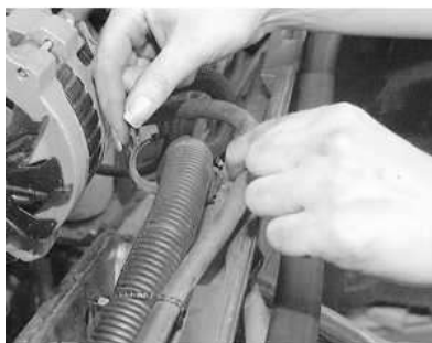
Fig. 1: Unclip the wiring harness retainer for access to the trim panel retainers
