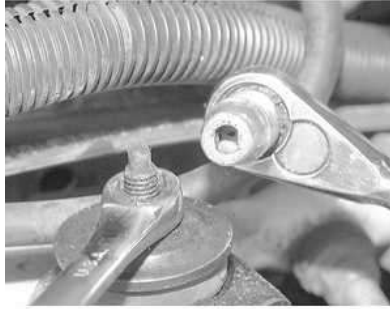
Fig. 5: Use a wrench to loosen the shock upper nut while holding the ratchet and socket over the shock stud
