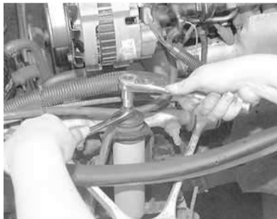
Fig. 5: Use a wrench to loosen the shock upper nut while holding the ratchet and socket over the shock stud
