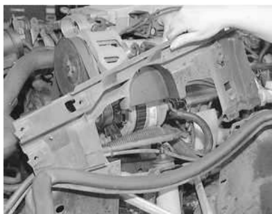
Fig. 2: Unfasten the trim panel retainers, then lift the panel up and out of the vehicle for access to the upper shock nut
