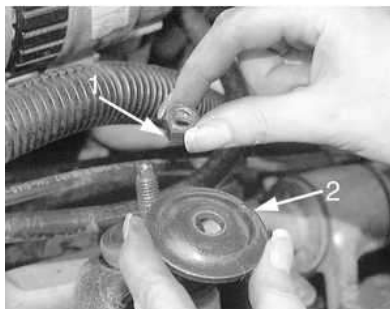
Fig. 6: Remove the upper shock mounting nut (1) and insulator retainer (2) . . .
