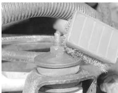
Fig. 3: Use a wire brush to clean off the upper shock mounting nut threads and stud
