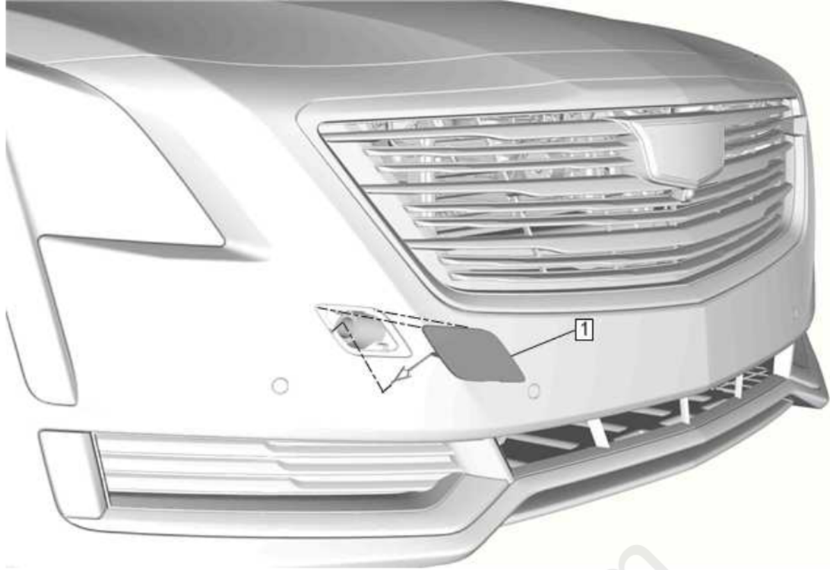
Fig. 3: Front Bumper Fascia Tow Eye Access Hole Cover Courtesy of GENERAL MOTORS COMPANY
