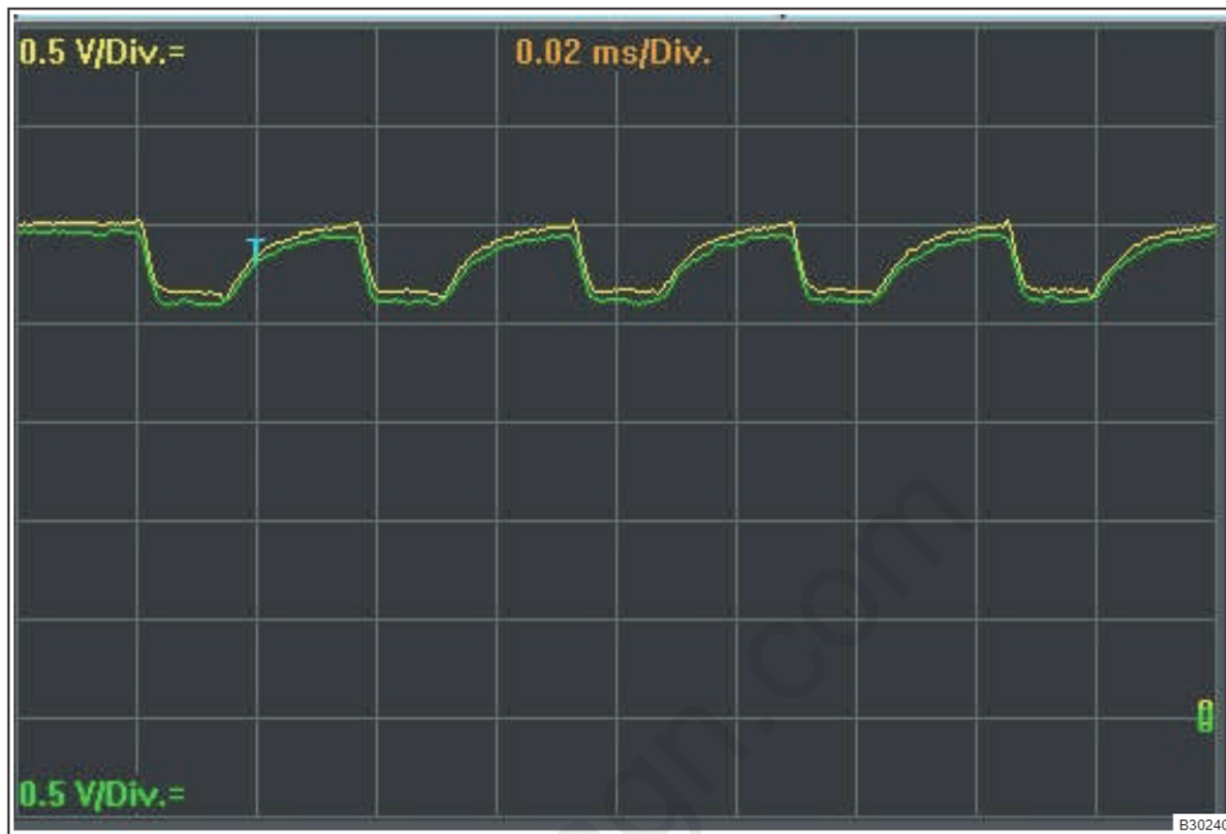
Short circuit malfunction waveform of CAN-H and CAN-L
