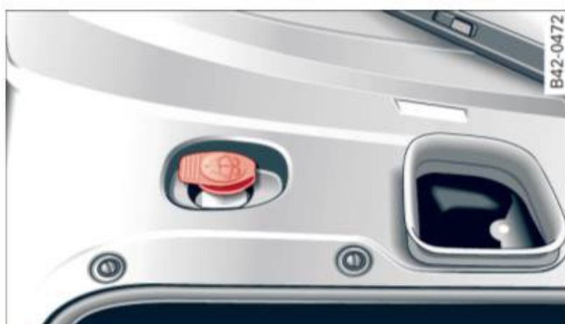
Fig. 147 Luggage compartment: Windshield washer fluid reservoir
