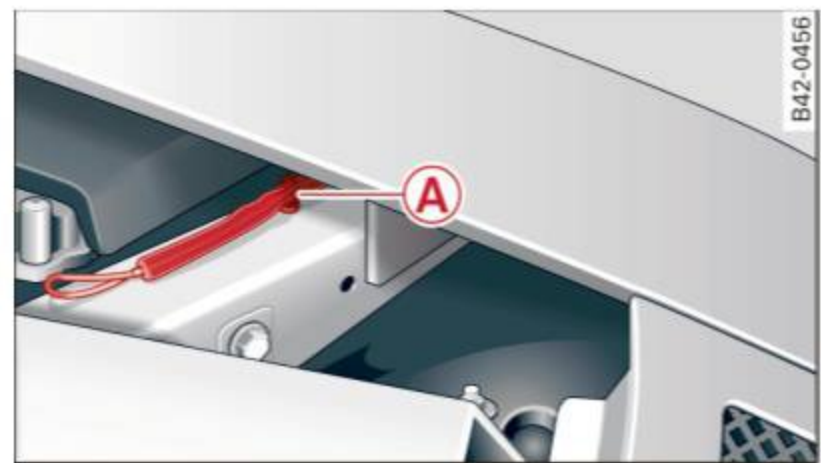
Fig. 135 Engine compartment: loosening the fuel filler flap cable
