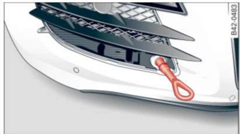
Fig. 162 Right front bumper without grille: Towing loop fully screwed in
