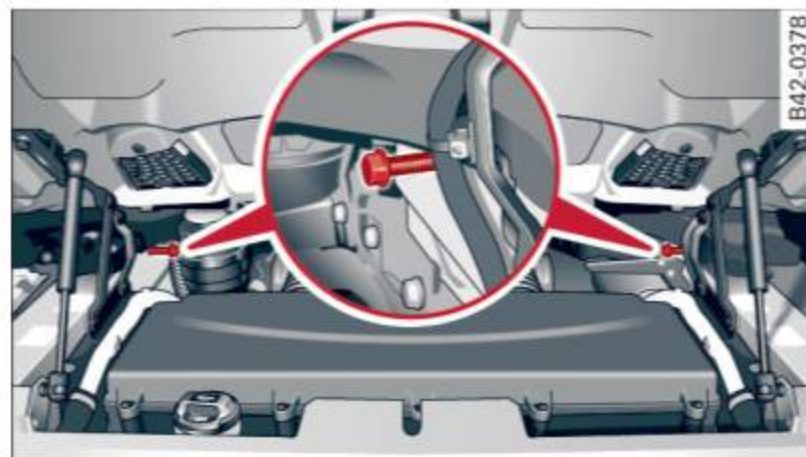
Fig. 47 Engine compartment: installing the emergency operation bolts
