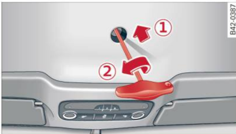
Fig. 56 Inner side of the convertible top: positioning the Allen wrench
