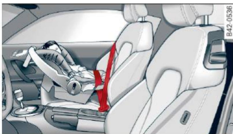
Fig. 128 Rearward-facing infant seat, properly installed on the passenger seat
