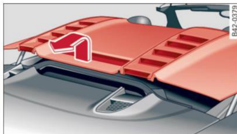
Fig. 48 Raising the storage bay lid and pulling it back
