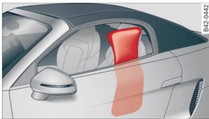
Fig. 127 Inflated side airbags on left side of vehicle
