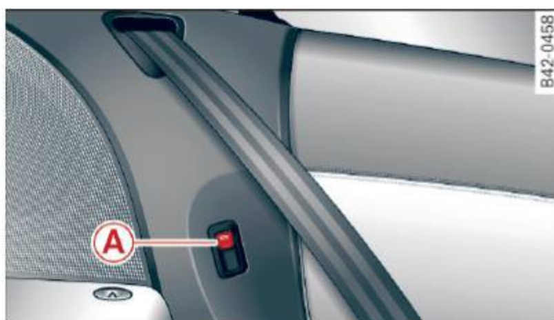
Fig. 137 Driver's side: releasing the engine compartment lid
