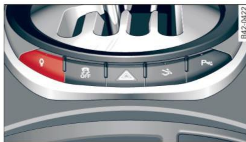
Fig. 85 Center console: Switch for Audi magnetic ride
