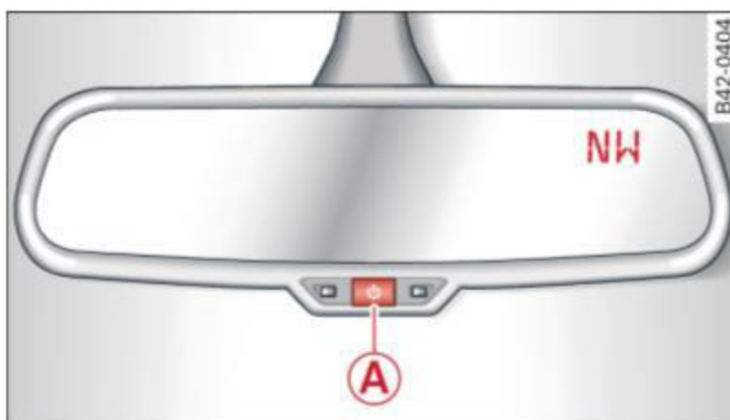
Fig. 71 Inside rearview mirror: digital compass activated
