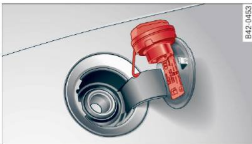
Fig. 134 Fuel cap hooked on the opened fuel filler flap
