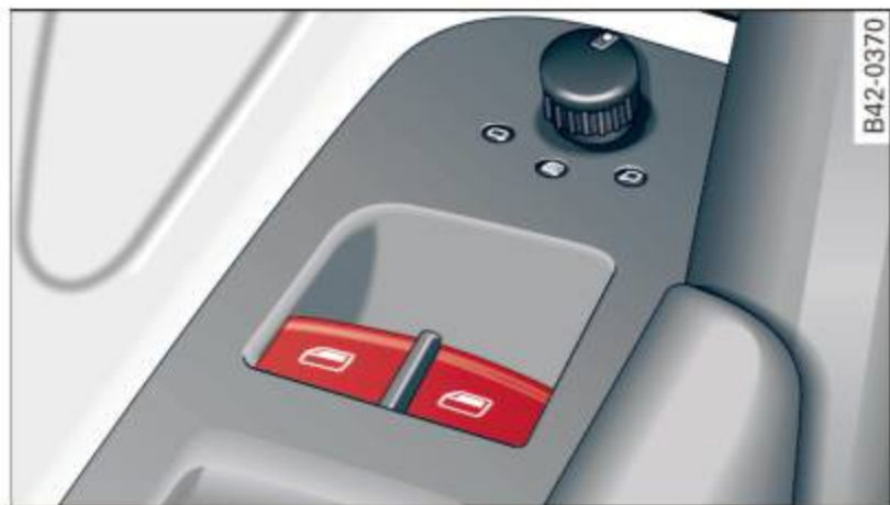
Fig. 38 Driver's door: power window switches
