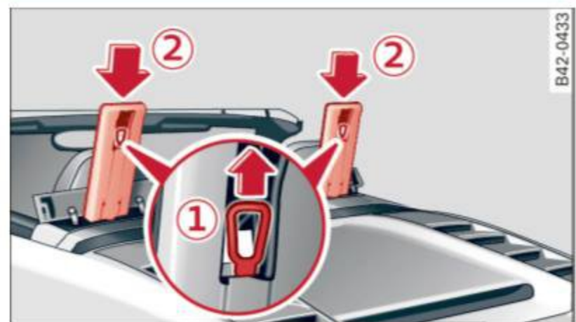
Fig. 108 Deployed rollbar with release loop
