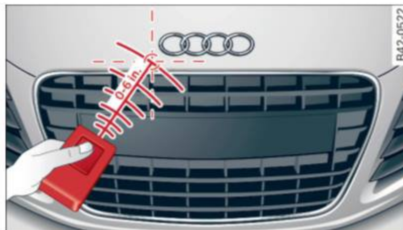
Fig. 102 Front bumper, driver side: location of transmitter unit
