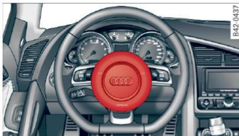
Fig. 120 Location of driver airbag: in steering wheel
