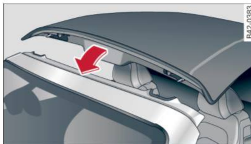
Fig. 52 Windshield frame: pressing the convertible top forward
