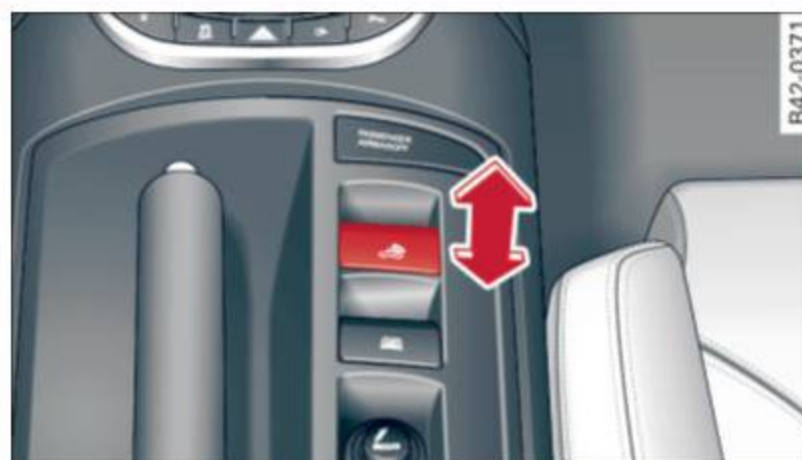
Fig. 40 Center console: convertible top switch
