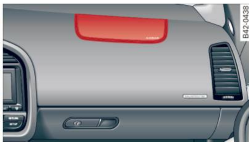
Fig. 121 Location of front passenger's airbag: in the instrument panel
