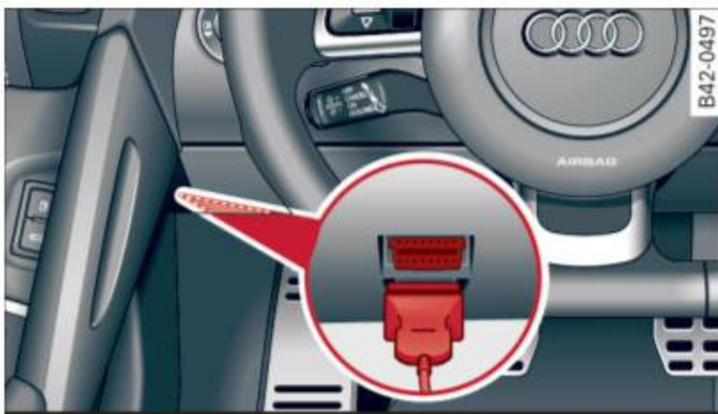
Fig. 9 Location of Data Link Connector (DLC)
