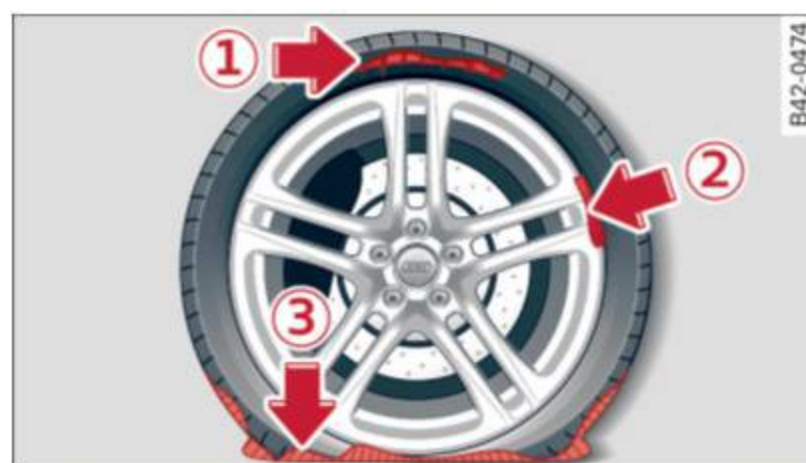
Fig. 153 Tire damage for which the Tire Mobility System is not suited
