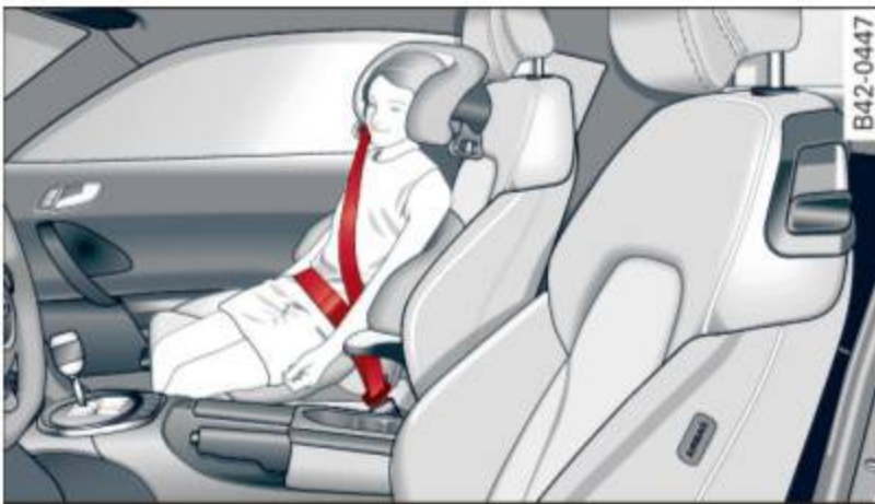
Fig. 130 Passenger seat: child properly restrained in a booster seat
