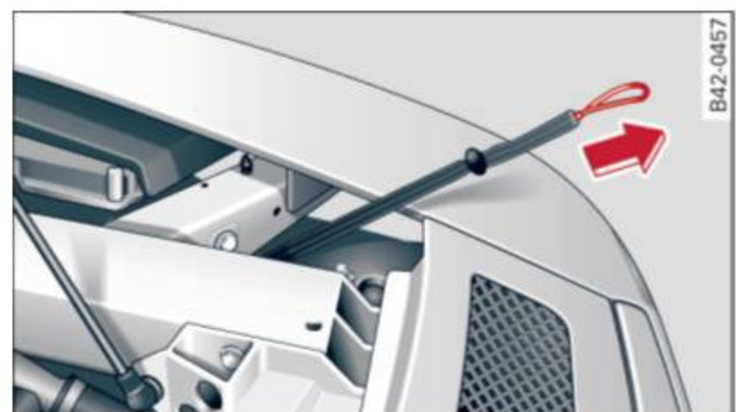
Fig. 136 Engine compartment: releasing the fuel filler flap using the emergency release
