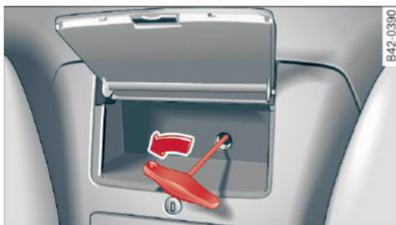
Fig. 59 Upper storage compartment between the seat backrests: extending the rear window
