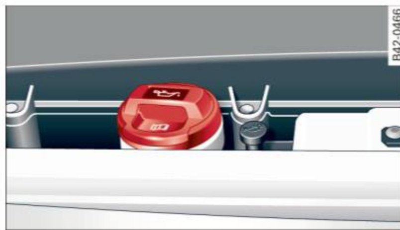
Fig. 142 Engine compartment: Oil filler cap location
