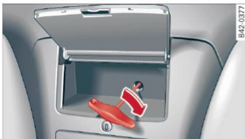
Fig. 46 Upper storage compartment: using the Allen wrench as a crank to lower the rear window
