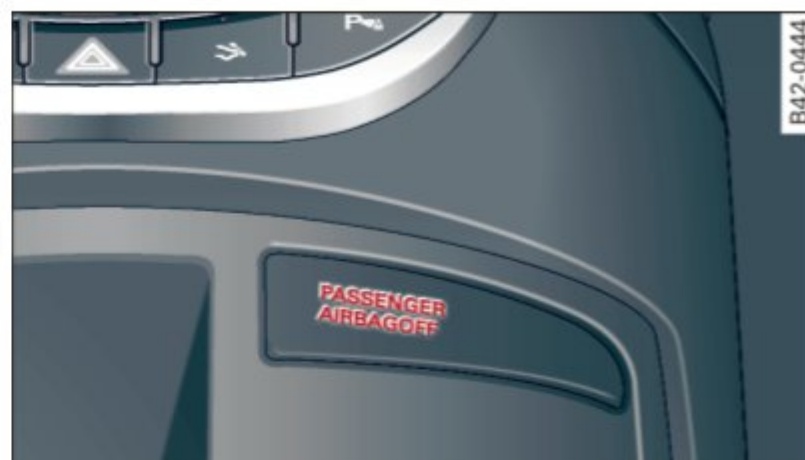
Fig. 123 Section from the instrument panel: PASSENGER AIR BAG OFF light
