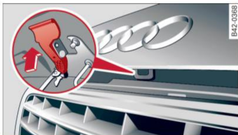
Fig. 35 Release lever under the front lid
