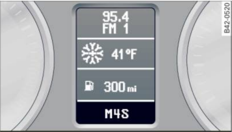
Fig. 88 Display: Gears engaged
