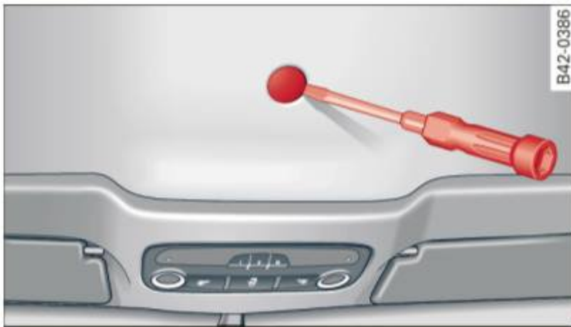
Fig. 55 Inner side of the convertible top: removing the cap
