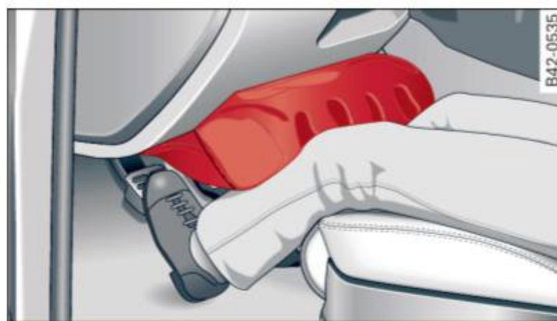
Fig. 125 Inflated airbags protecting in a frontal collision
