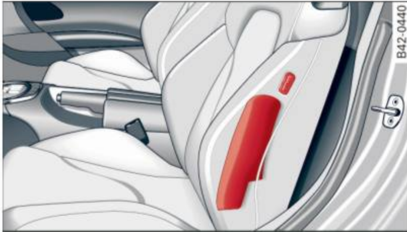
Fig. 126 Side airbag location in the driver's seat
