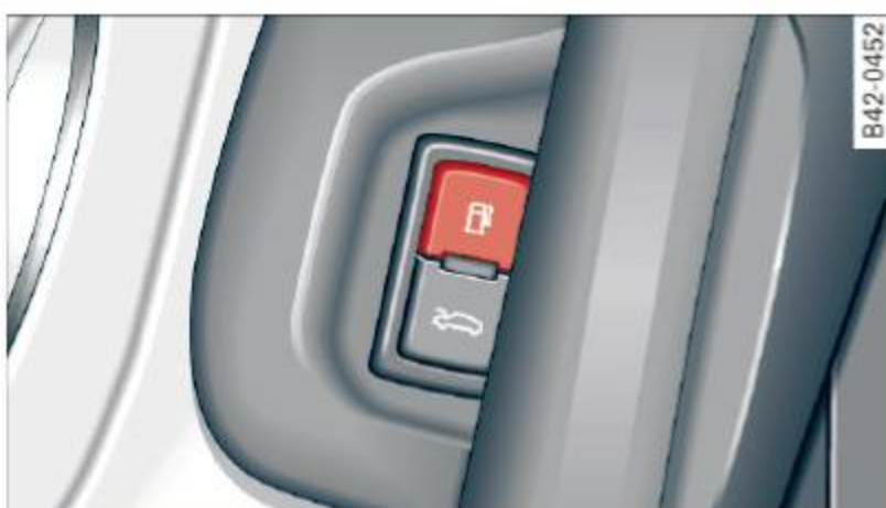
Fig. 133 Driver's door: Unlocking fuel filler flap
