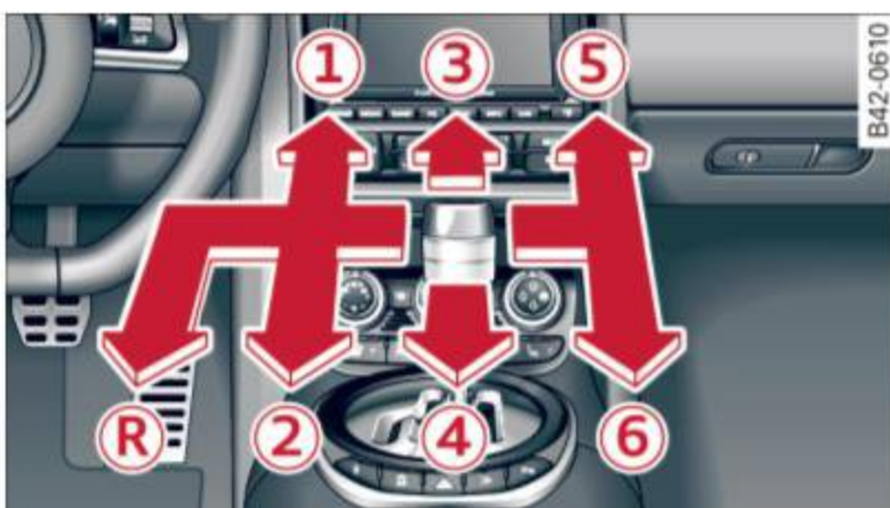
Fig. 86 Gearshift pattern: 6-speed manual transmission
