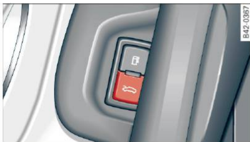
Fig. 34 Drivers door: remote front lid release
