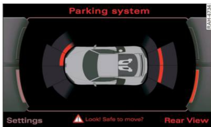
Fig. 95 Navigation system display: visual distance display
