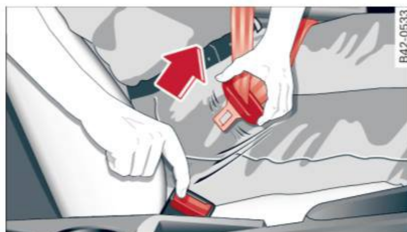
Fig. 119 Releasing the tongue from the buckle
