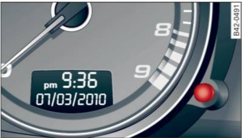
Fig. 25 Section of instrument cluster: Set/Check button
