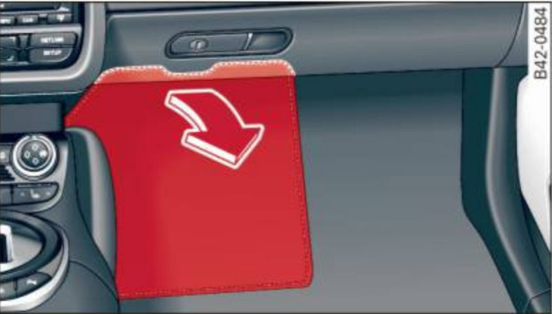
Fig. 163 Passenger's side wheel well: Foot rest with fuse arrangement
