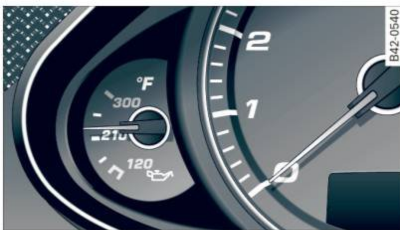
Fig. 140 Instrument cluster: Engine oil temperature display
