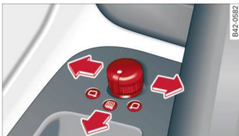
Fig. 70 Forward section of driver's armrest: power mirror controls
