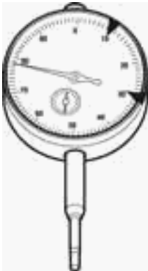
VAS 6079 Dial gauge For setting TDC of the 1st cylinder
