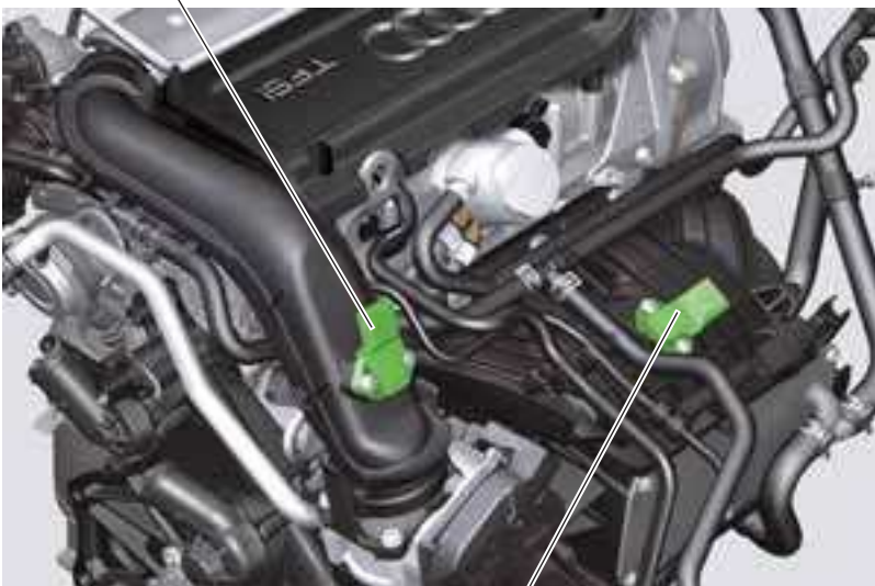
Intake manifold pressure sender G71 with intake air temperature sensor G42
