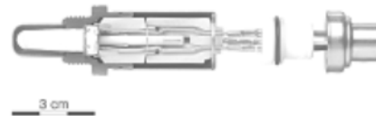
Interior structure of oxygen sensor
