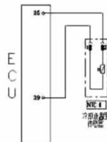
Circuit diagram of Coolant temperature sensor
