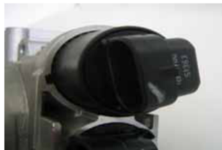
Idle actuator with step motor
