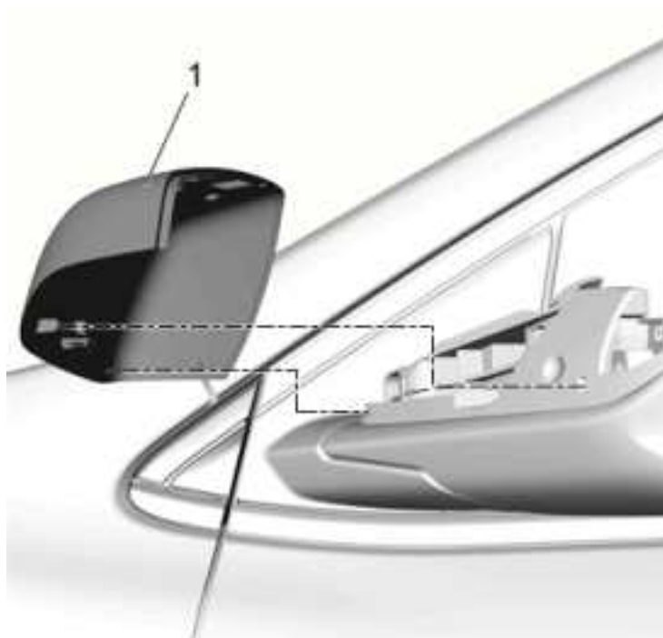
Fig. 10: Outside Rearview Mirror Housing Upper Cover
