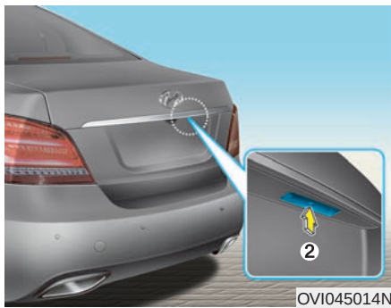
(2) Power Trunk Open button
