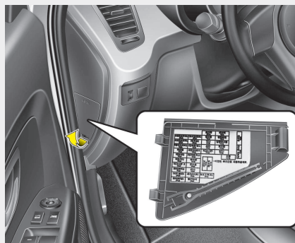
Inner fuse panel
