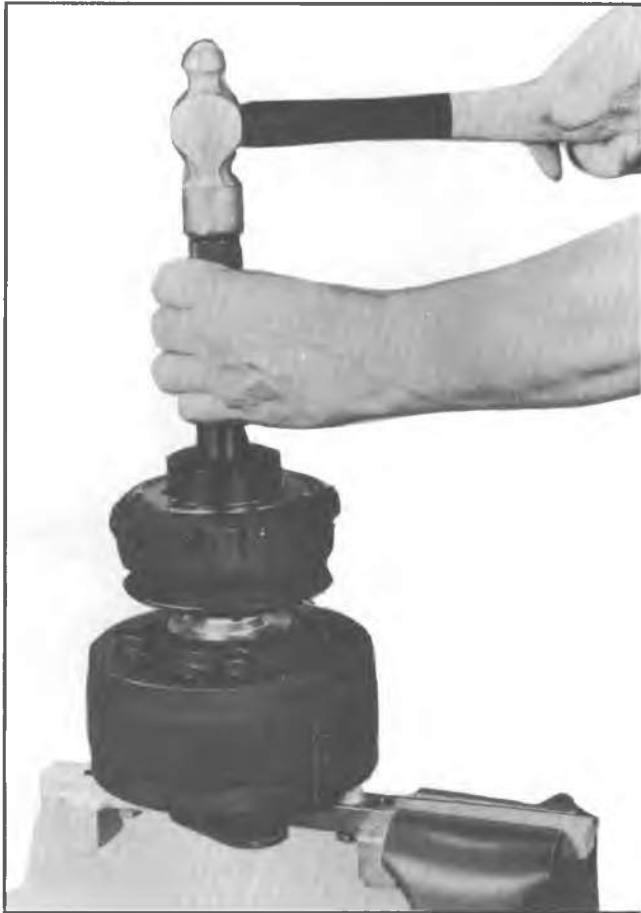
Fig. 84--Alternate Installation of R-4 Rotor and Bearing Assembly
