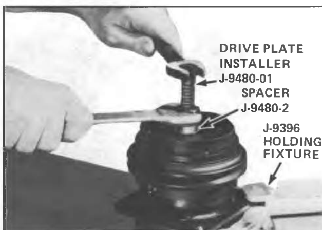
Fig. 8--Installing Drive Plate
