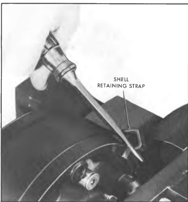
Fig. 90--Releasing Retaining Strap
