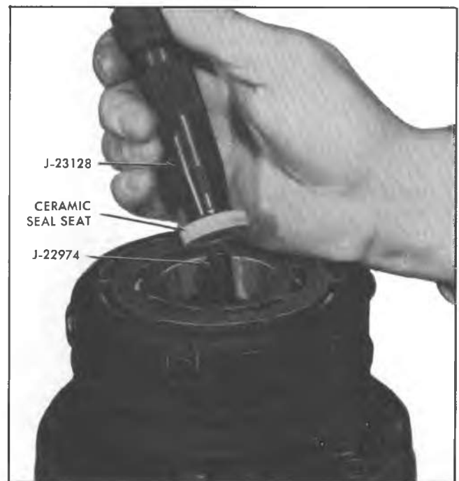
Fig. 73--Removing Seal Seat
