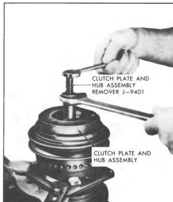
Fig. 4--Removing Clutch Plate and Hub Assembly
