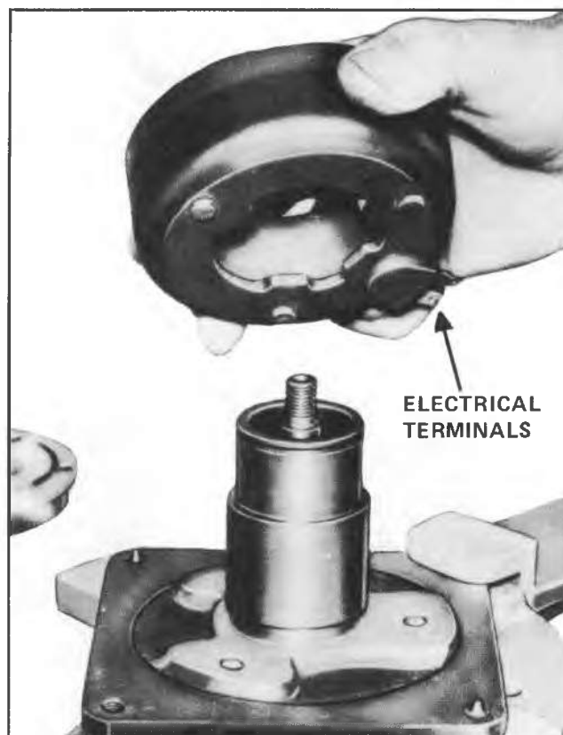
Fig. 17--Installing Coil Housing
