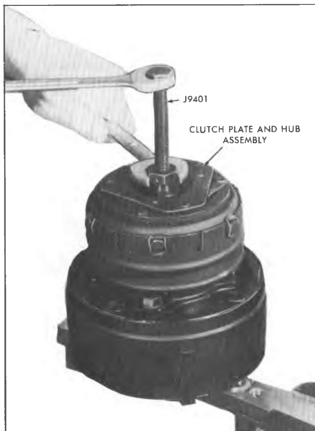
Fig. 70--Removing Clutch Plate and Hub Assembly
