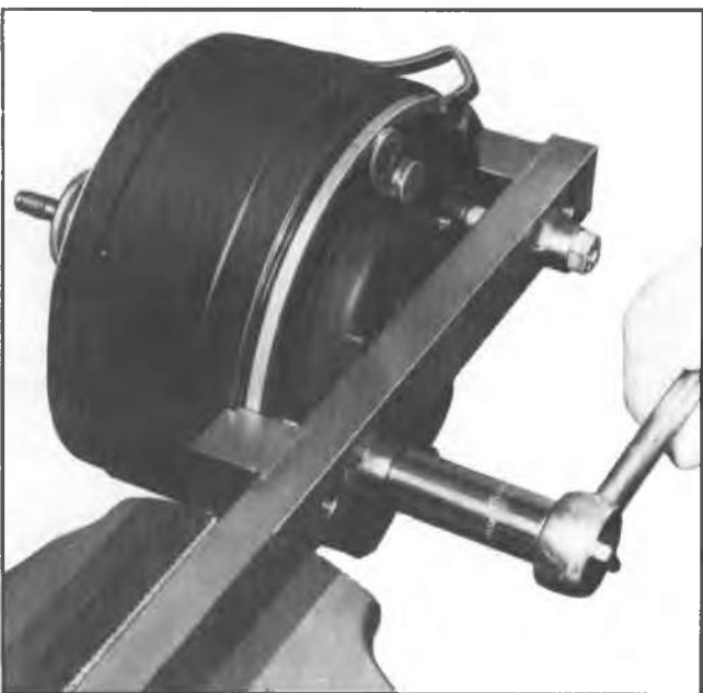
Fig. 91--Removing Shell Assembly
