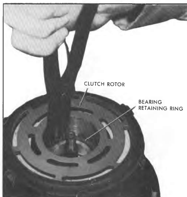
Fig. 76--Removing Bearing Retaining Ring
