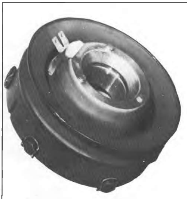
Fig. 79--Clutch Coil and Housing Assembly
