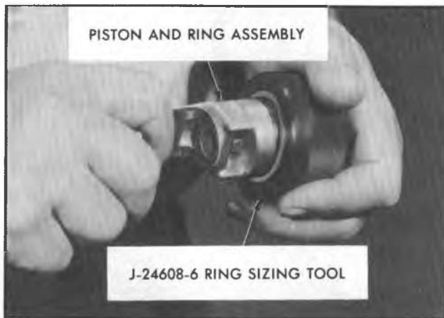
Fig. 48--Turning Piston and Ring Asm. into Ring Sizing Tool
