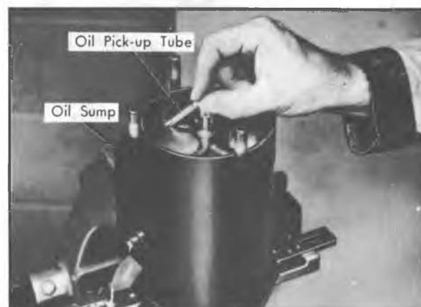
Fig. 63--Installing Oil Pick-Up Tube
