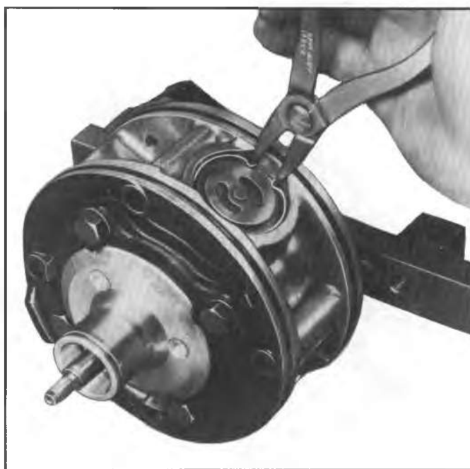
Fig. 92--Removing Valve Plate
