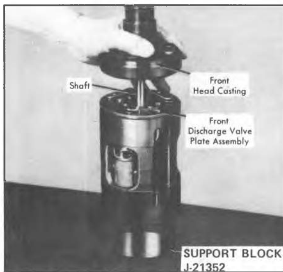
Fig. 60--Installing Front Head Casting
