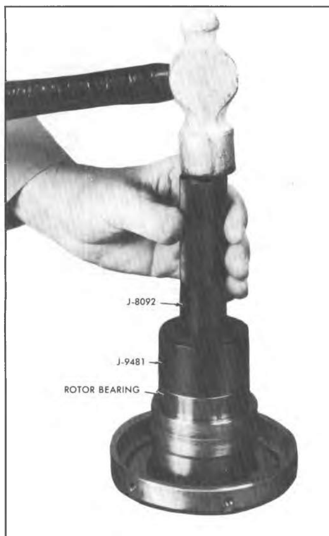
Fig. 82--Installing Clutch Rotor Bearing
