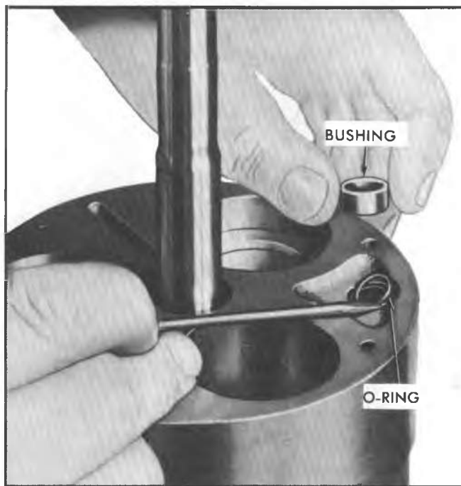
Fig. 56--Installing O-Ring On Discharge Cross-over Tube
