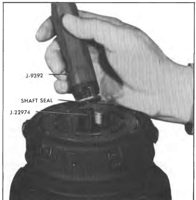
Fig. 74--Removing Shaft Seal
