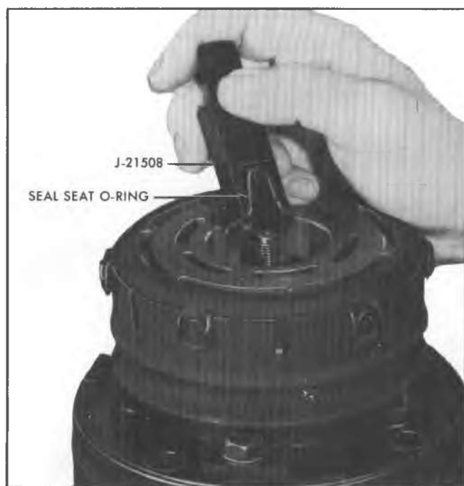
Fig. 75--Installing Seal Seat "O" Ring
