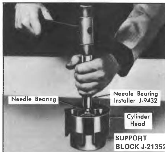
Fig. 35--Installing Needle Bearing
