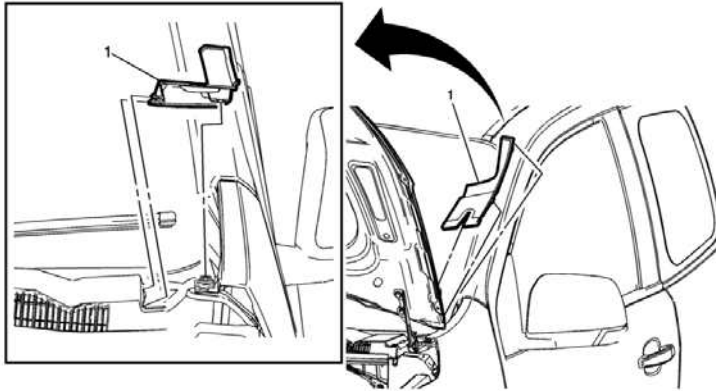
Air Inlet Grille Panel Extension Replacement
