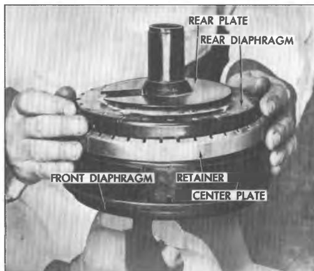
Fig. 5-11B--Installing Rear Diaphragm Retainer
