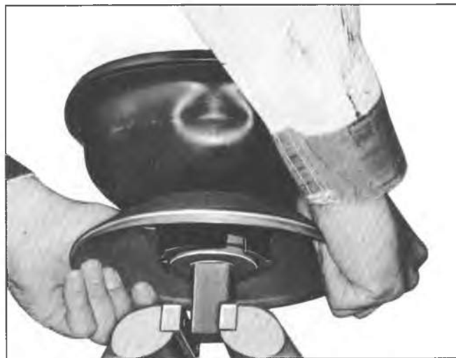
Fig. 5-9C--Positioning Power Piston on Support Plate Remover
