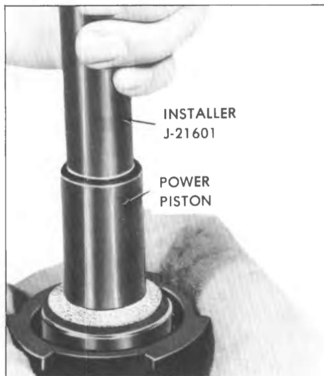
Fig. 5-13C--Installing Floating Control Valve Assembly
