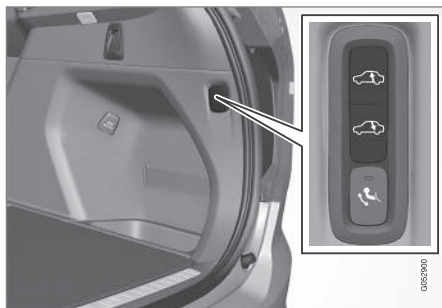
Level control buttons on the rear edge of the cargo compartment
