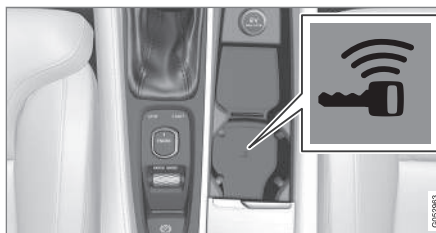
Back-up reader in the tunnel console
