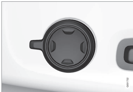
Multifunction control on the side of the seat
