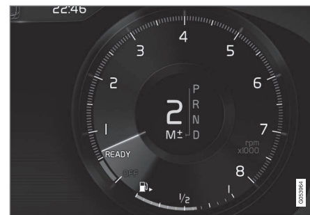
Instrument panel when the paddles are activated
