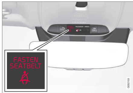
Seat belt reminder light in ceiling console
