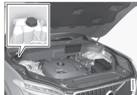
Coolant expansion tank
