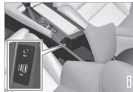
AUX/USB sockets in the tunnel console
