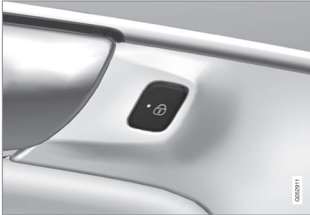
Rear door lock button and indicator light
