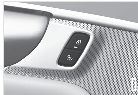
Front door lock button and indicator light
