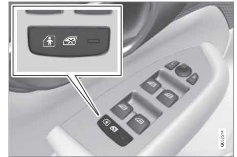
Child safety lock button on the driver door control panel
