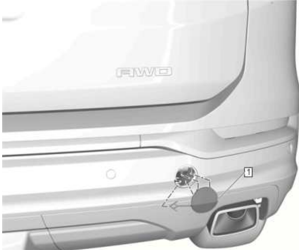
Fig. 24: Rear Bumper Fascia Tow Eye Access Hole Cover (Terrain).
