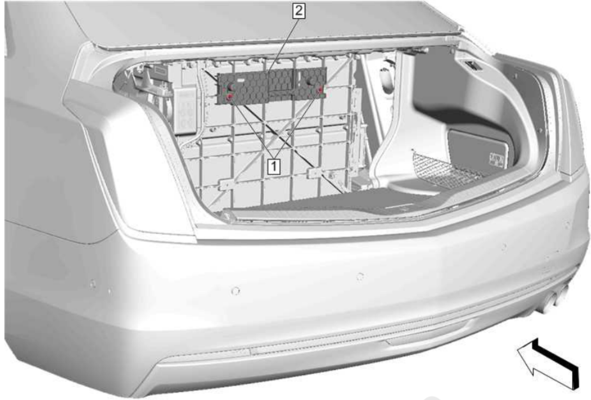
Fig. 181: High Voltage Battery Cover Bracket Courtesy of GENERAL MOTORS COMPANY
