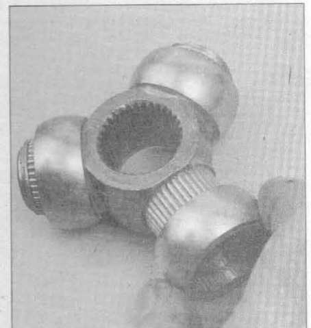
11.3k Clean all of the old grease out of the housing and spider assembly, then remove each bearing, one at time
