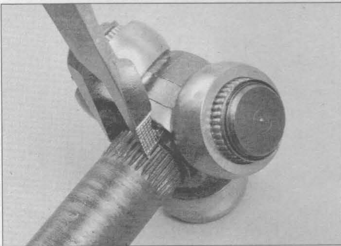
11.3e If the spider is positioned by a stop ring, spread the ends of the stop ring apart and slide it towards the center of the shaft
