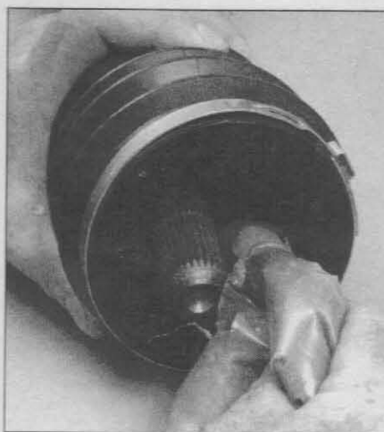
11.4r Install the small clamp and the boot on the driveaxle and apply grease to the inside of the axle boot until ...
