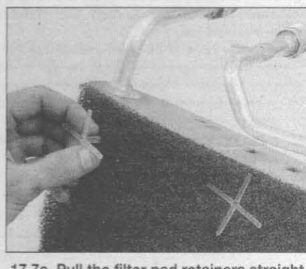
17.7a Pull the filter pad retainers straight out and lift the filter pad from the evaporator core
