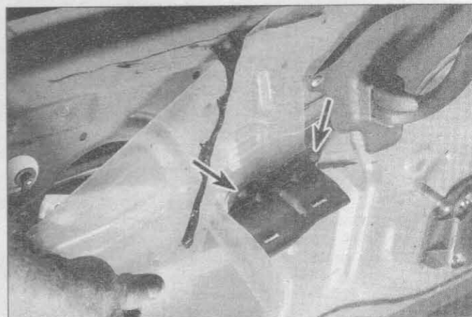
15.8b To get at the inner door components, simply peel off the deflector in the area in which you need to work; if you need to remove the entire deflector, drill out the two rivets (arrows) for the armrest hanger and remove the hanger
