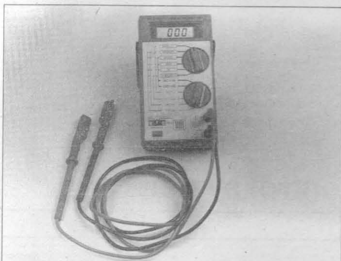
2.1 Digital multimeters can be used for testing all types of circuits; because of their high impedance, they are much more accurate than analog meters for measuring millivolts in low-voltage computer circuits
