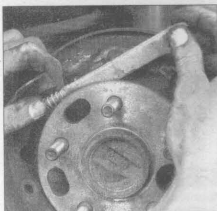
6.4e Spread the shoes apart at the top and remove the parking brake strut
