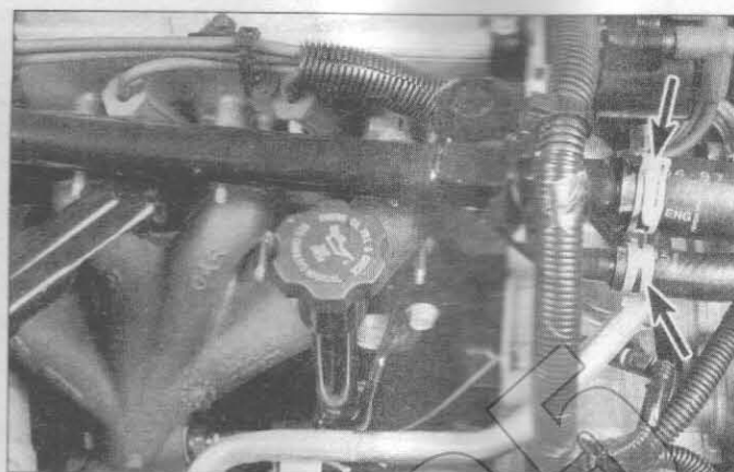
8.9 Remove the mounting clamps (arrows) and separate the heater outlet hoses from the pipes
