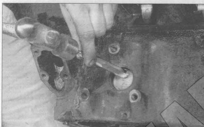
16.4a A hammer and large punch can be used to knock the core plugs sideways in their bores
