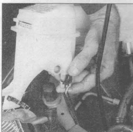
5.19 Lift the coolant reservoir from the engine compartment and disconnect the coolant level sensor connector
