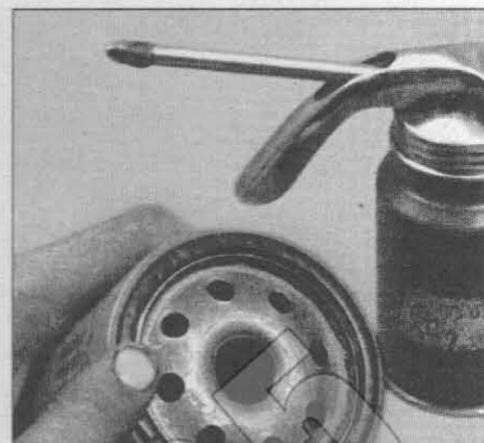
9.14 Lubricate the oil filter gasket with clean engine oil before installing the filter on the engine
