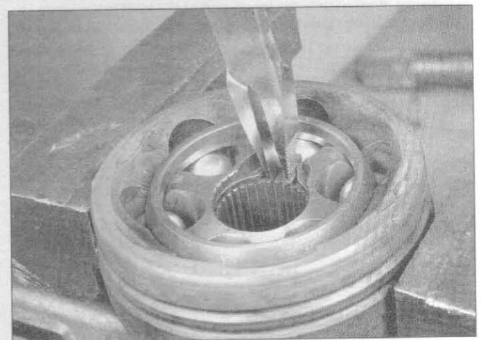
11.4p ... then seat it into the groove with snap-ring pliers
