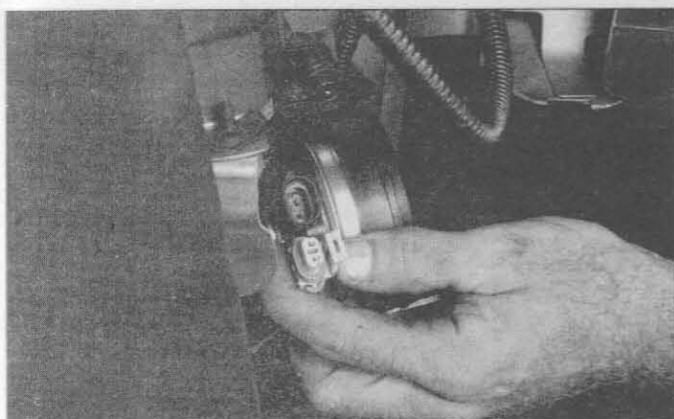
21.2 To test the horn, connect the horn to the battery with fused jumper wires; if the horn doesn't operate, replace it
