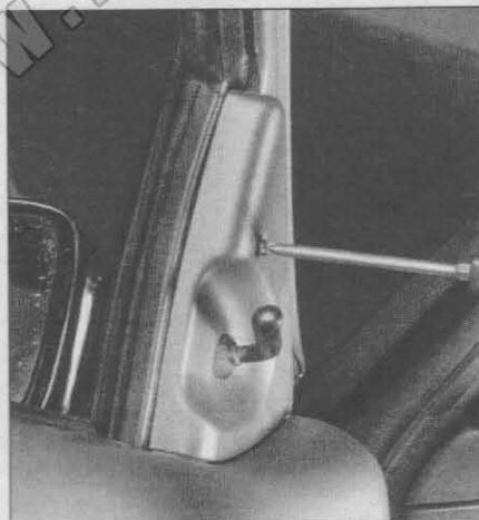
20.2a To get to the outside mirror retaining nuts, remove this Phillips screw...
