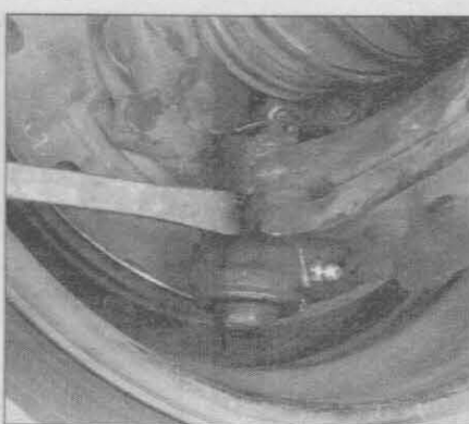
6.3b With the prybar positioned between the steering knuckle boss and the balljoint, pry down and check for play in the balljoint - if there's any play, replace the balljoint
