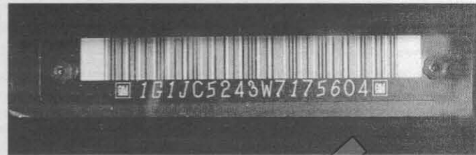
The Vehicle Identification Number (VIN) is stamped into a metal plate fastened to the dashboard on the driver's side - it's visible through the windshield
