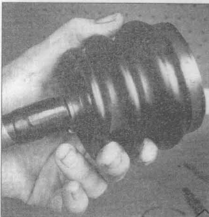
11.3n Wrap the axle shaft splines with tape to avoid damaging the boot, then slide the small clamp and boot onto the axle shaft
