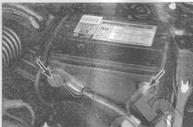
11.4 Check the tightness of the battery cable terminal bolts (arrows)
