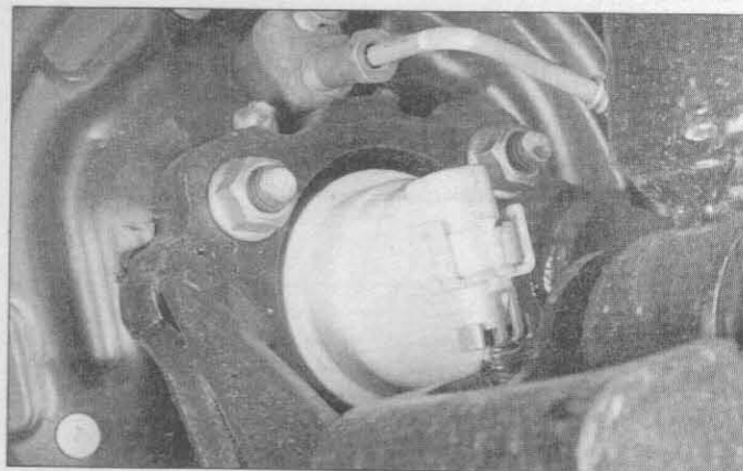
2.4b The rear wheel speed sensors are mounted in the rear drum brake backing plates; the toothed rings (not visible in this photo) are installed on the inner side of the flange for each hub and bearing unit
