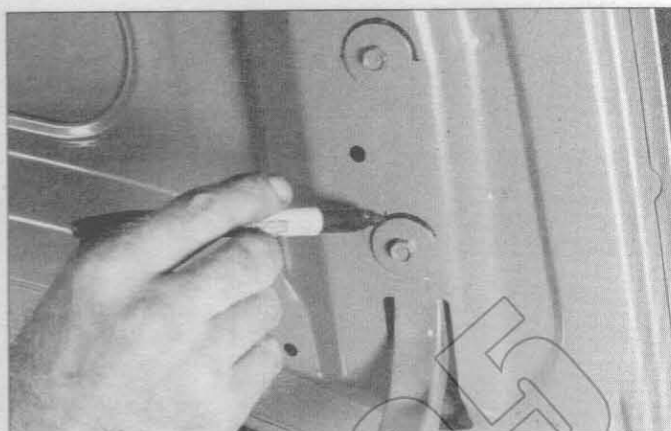
13.3 Before removing the four (two per side) trunk lid hinge bolts, be sure to mark the relationship of the hinge to the trunk lid to ensure correct alignment when the lid is installed
