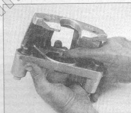
4.16 Lubricate the piston bore and seal with clean brake fluid before installing the new seal in the caliper bore groove
