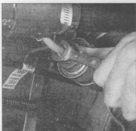
26.5b Loosen the fuel line fitting with a flare-nut wrench - be sure to use an open-end wrench on the filter as a back-up
