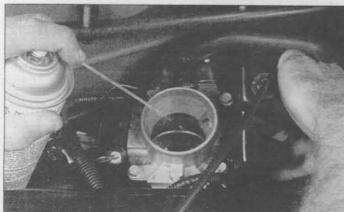
13.2 Spray carburetor cleaner into the throttle body to break away any carbon deposits or sludge that may have collected around the throttle plate
