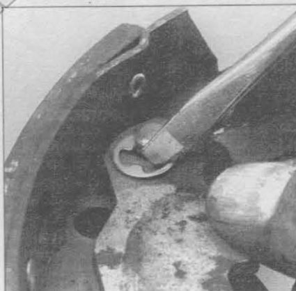
6.4i Remove the parking brake lever by prying off the C-clip
