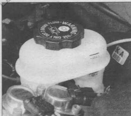
4.18 The fluid level inside the brake fluid reservoir can easily be checked by observing the level from the outside - fluid can be added to the reservoir after the cover is removed by prying up on the tabs
