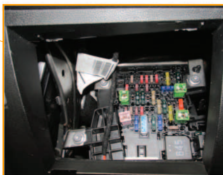
Relay and fuse holder SC at the bottom left of the passenger compartment, behind the storage compartment
