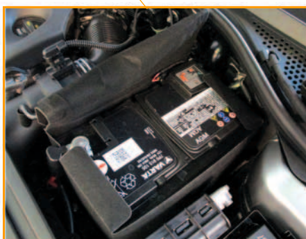
12V battery in engine compartment
