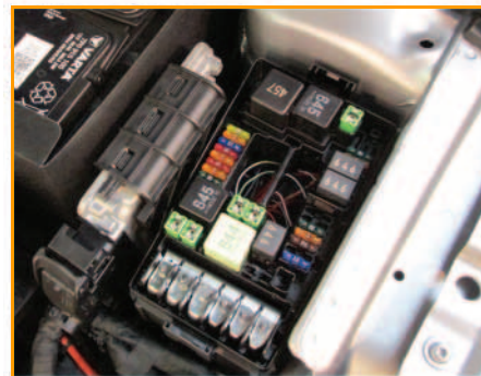
Electronics box with relay and fuse holder SB and multifuse pre-fuse holder SA
