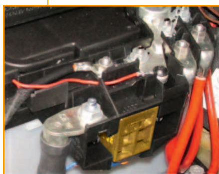
Main fuse box with fuse holder SD, positive battery terminal clamp and battery isolator switch J990
