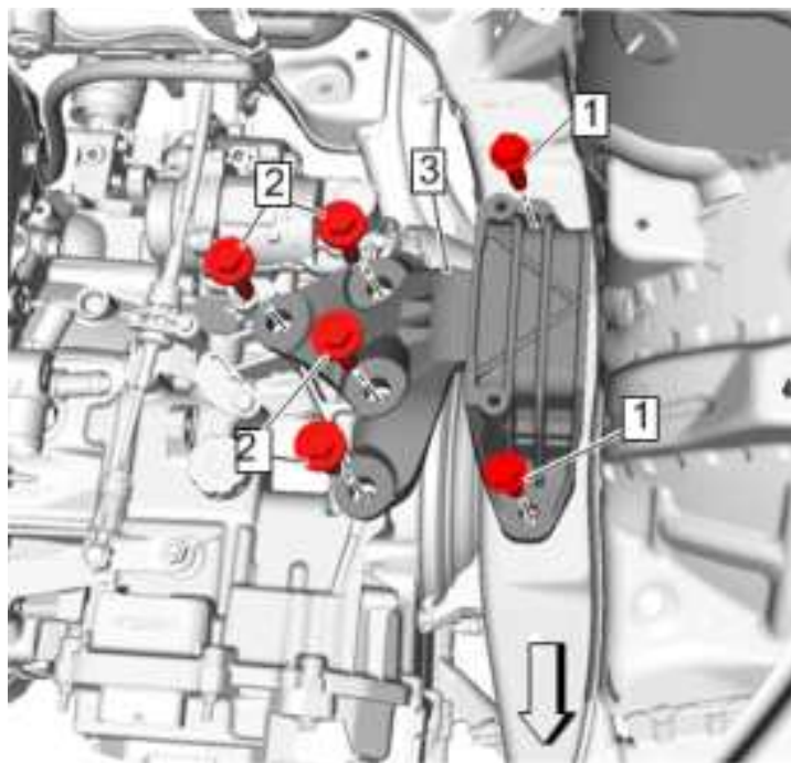
Fig. 39: Bolts At Left Transmission Mount
