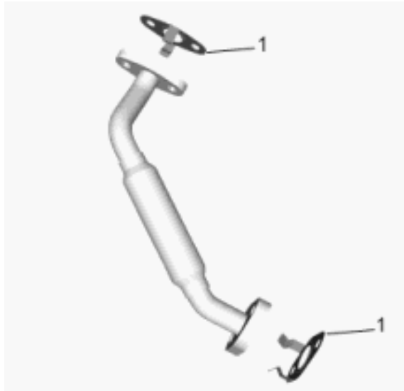
Fig. 60: Turbocharger Oil Return Pipe Gaskets Courtesy of GENERAL MOTORS COMPANY
