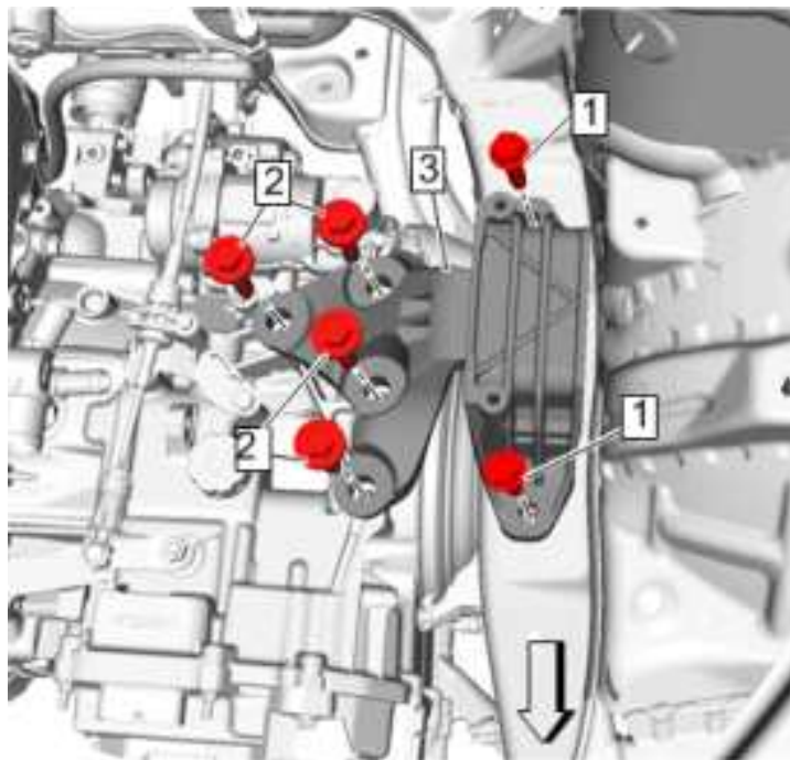
Fig. 37: Bolts At Left Transmission Mount
