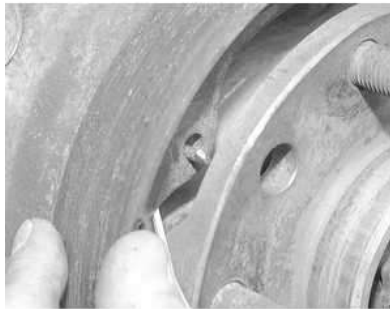
Fig. 12: Carefully place the shoe and lining assembly over the hold-down pins, being careful not to knock them out of the mounting holes
