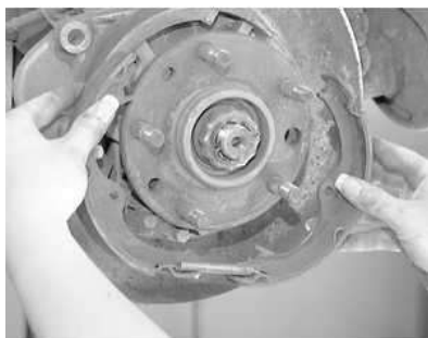
Fig. 5: Pull the shoe and linings apart enough to clear the hub and bearing, then remove the linings with the shoe return spring still engaged
