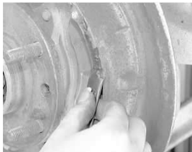
Fig. 10: Apply a small amount of a suitable silicone grease to the parking brake shoe wear shim contact areas
