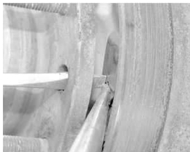
Fig. 3: Use a screwdriver to depress the hold-down spring, then slide the pin until it can be removed
