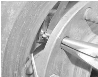
Fig. 13: Place the hold-down spring over the pin, and while holding the spring in place with a screwdriver, use needle-nose pliers to turn the pin to the secured position
