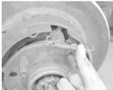
Fig. 2: Unhook and remove the adjuster return spring
