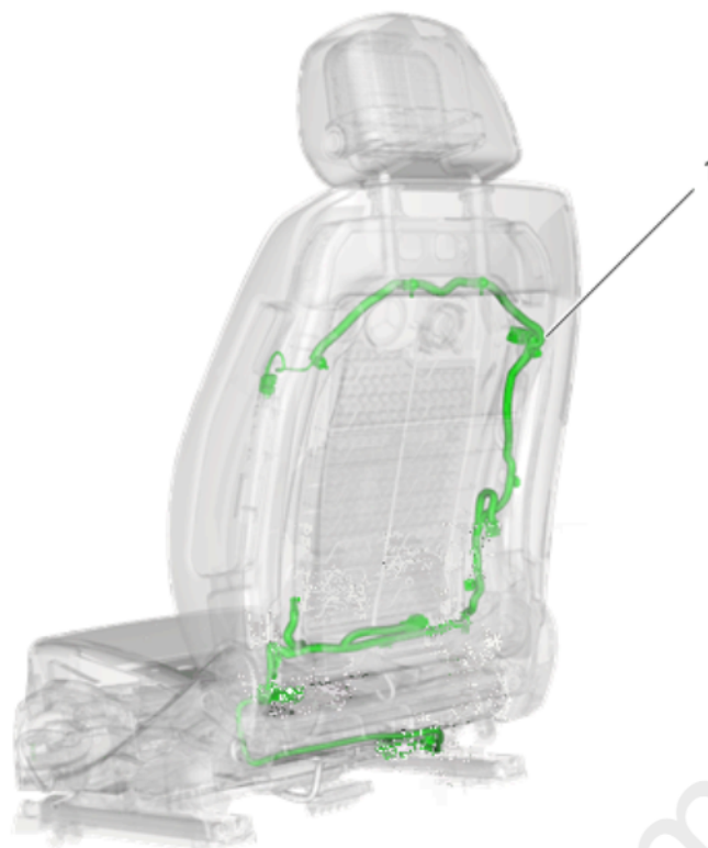
Fig. 21: Front Seat Back Wiring Harness Courtesy of GENERAL MOTORS COMPANY
