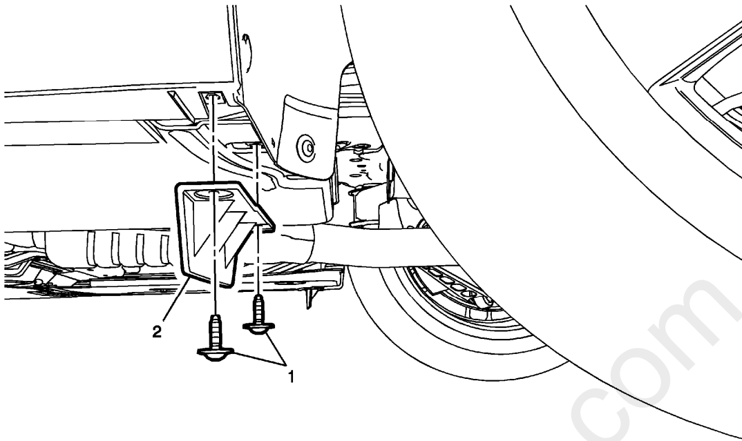
Fig. 82: Rear Tire Front Air Deflector Courtesy of GENERAL MOTORS COMPANY
