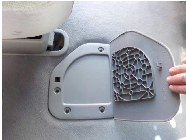
Hatch lifted. It just covers the screws.
