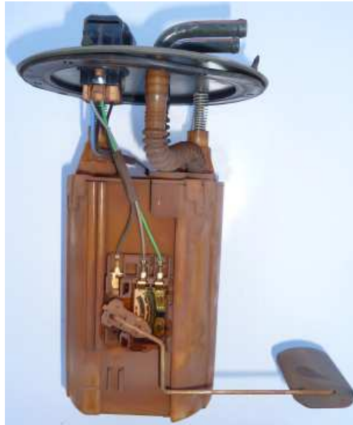
Photo showing the float, arm and sender mechanicals and electronics on the side of the canister can be seen. This is pictured as if taken from the front of the vehicle (i.e. the float arm points to the left of the vehicle).
