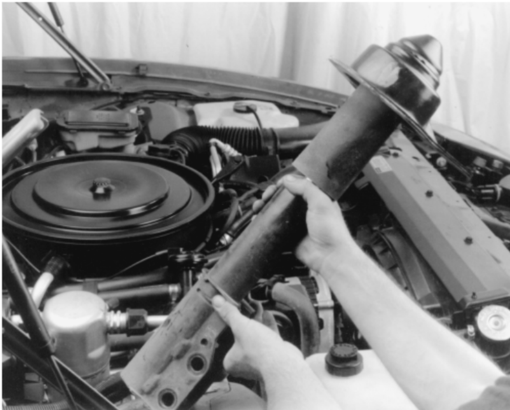
Fig. 4: Lifting out the strut
