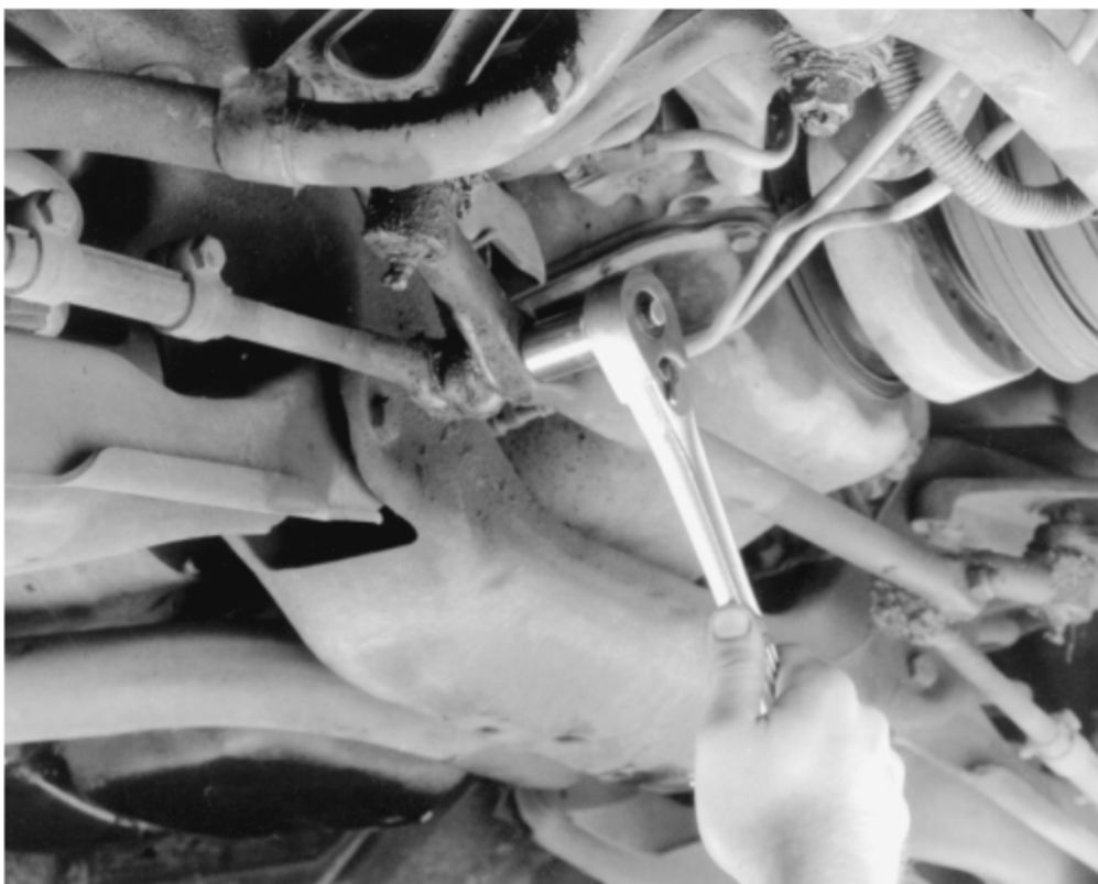
Fig. 4: Separating the tie rod from the relay rod using a gear puller
