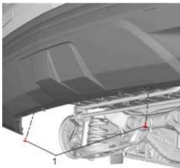
Fig. 79: Rear Bumper Fascia Lower Bolt
