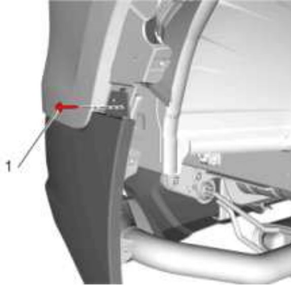
Fig. 86: Liftgate Bumper Pad Bolt Courtesy of GENERAL MOTORS COMPANY
