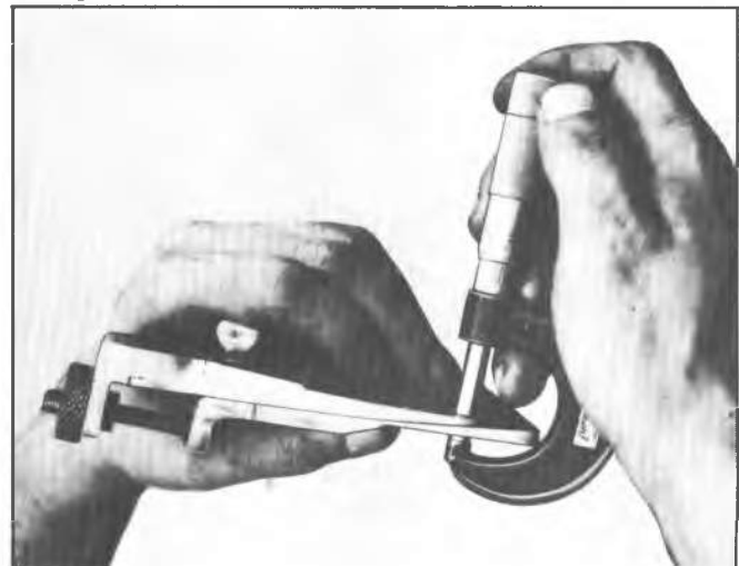
Fig. 10C—Measuring Gauge Plate Thickness
