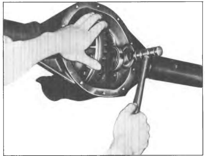
Fig. 9B—Installing Differential Shim
