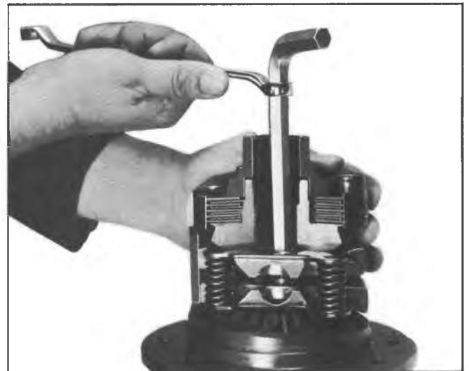
Fig. 5D—Removing Preload Spring Pack (Corvette)
