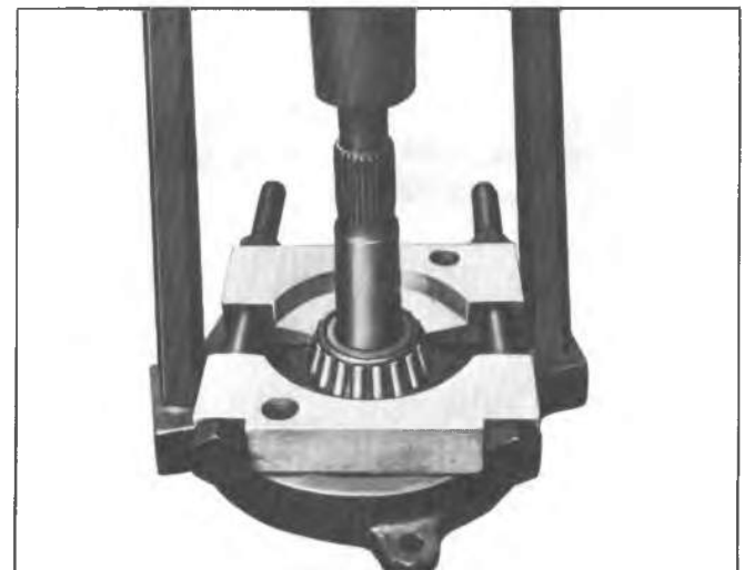
Fig. 4B-16--Removing Drive Pinion Rear Bearing Typical
