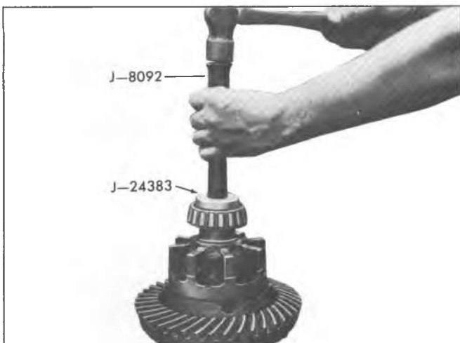
Fig. 7F—Installing Side Bearing
