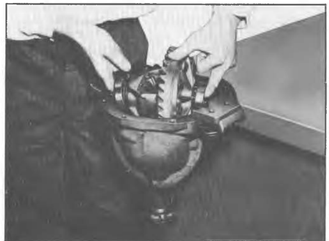
Fig. 8C—Installing Differential Assembly
