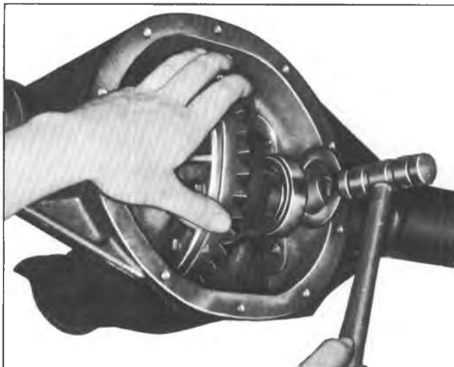
Fig. 4B-10--Installing Differential Shim
