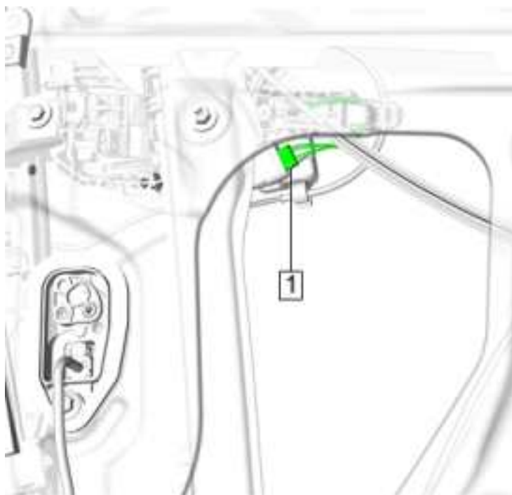
Fig. 72: Electrical Connector Courtesy of GENERAL MOTORS COMPANY
