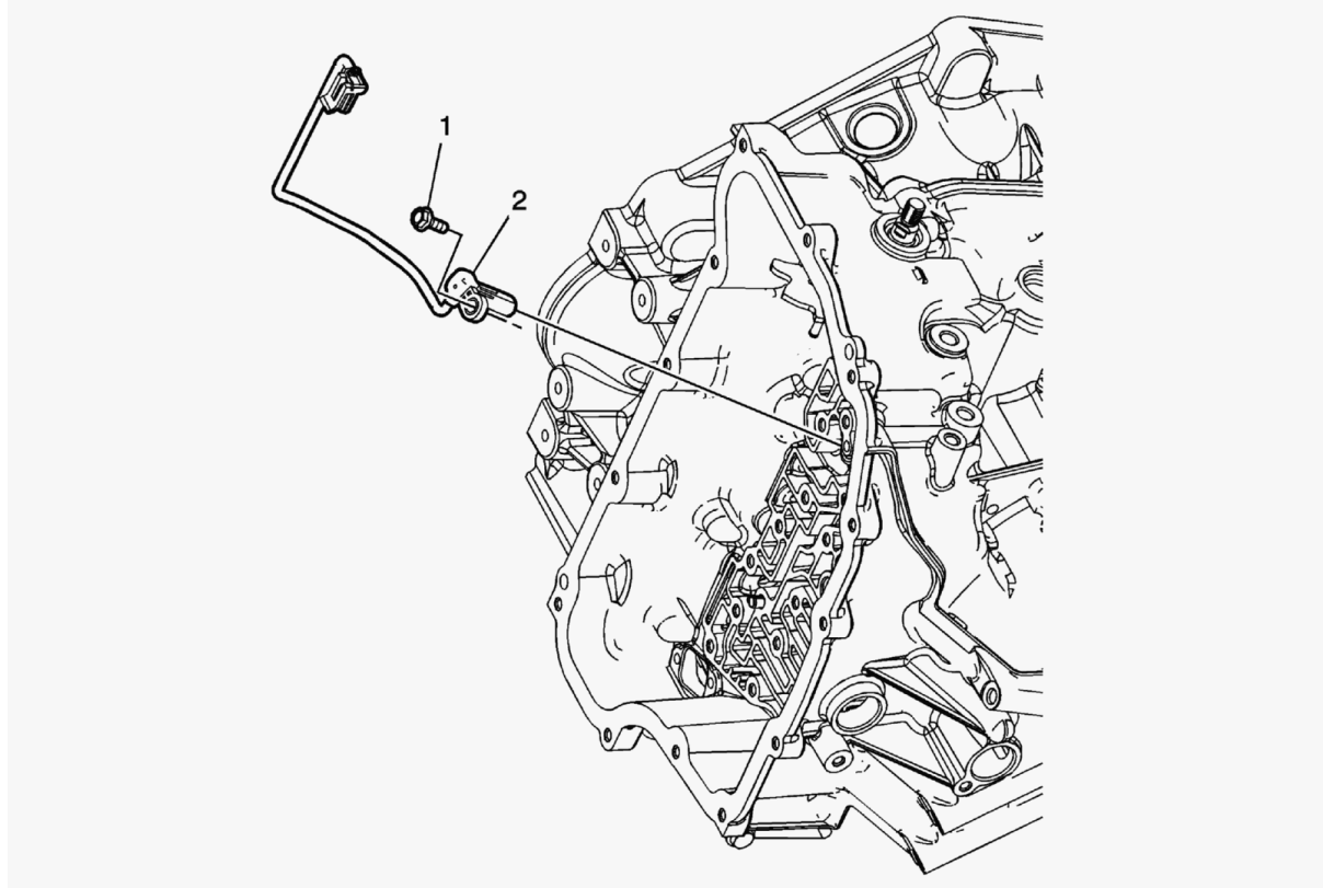
Fig. 76: Identifying Output Speed Sensor Courtesy of GENERAL MOTORS COMPANY
