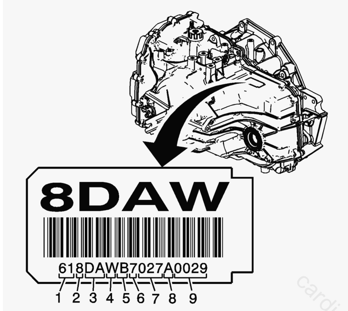
Fig. 1: Identifying Transmission Identification Information Plate
