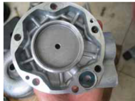
Inside structure of the compressor3
