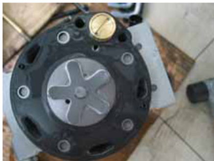
Inside structure of the compressor 2
