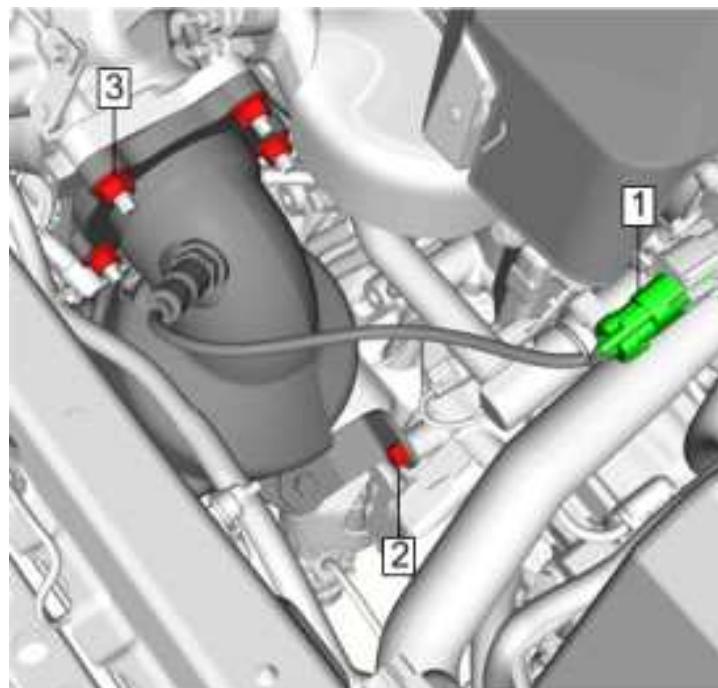
Fig. 55: Heated Oxygen Sensor Electrical Connector Courtesy of GENERAL MOTORS COMPANY
