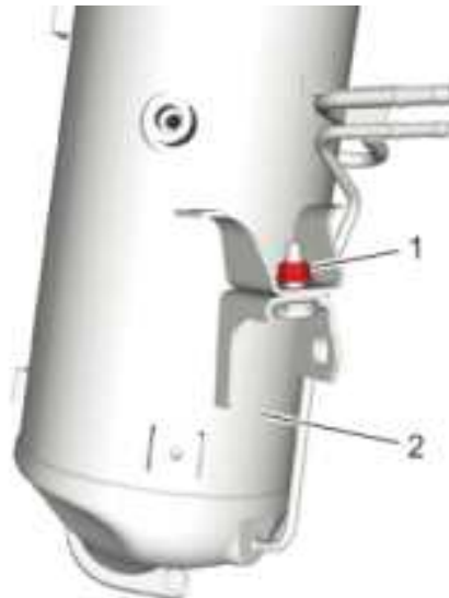
Fig. 37: Catalytic Converter Brace Bracket Nut Courtesy of GENERAL MOTORS COMPANY
