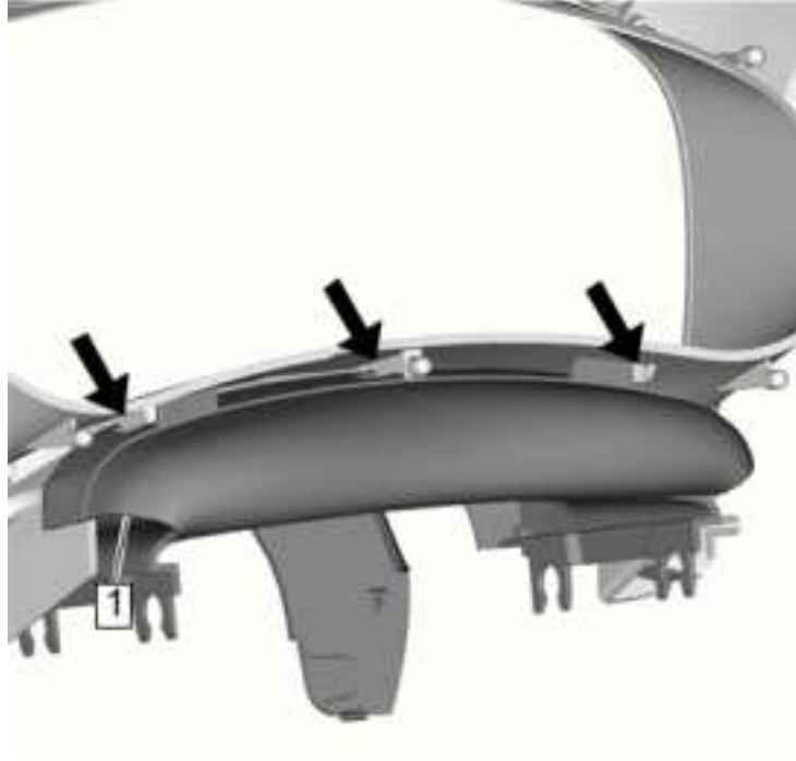
Fig. 250: Steering Column Upper Trim Cover Closeout Courtesy of GENERAL MOTORS COMPANY
