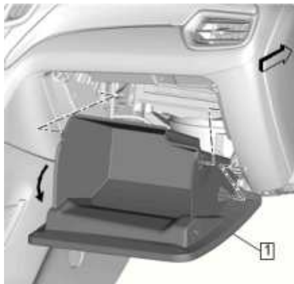
Fig. 329: Squeeze Sides Of Instrument Panel Compartment Door Courtesy of GENERAL MOTORS COMPANY
