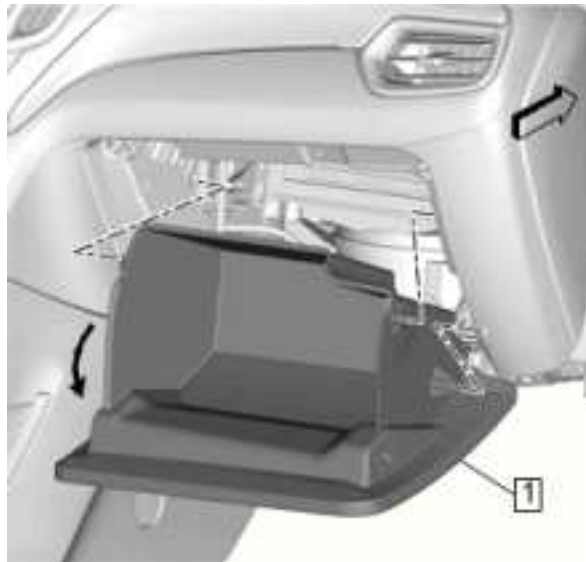
Fig. 319: Squeeze Sides Of Instrument Panel Compartment Door Courtesy of GENERAL MOTORS COMPANY
