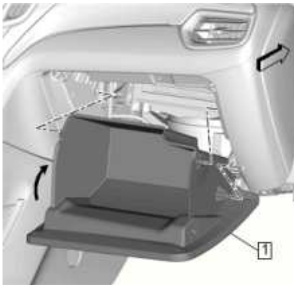
Fig. 322: Squeeze Sides Of Instrument Panel Compartment Door Courtesy of GENERAL MOTORS COMPANY
