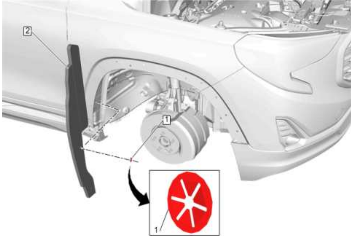
Fig. 72: Front Fender Insulator (Right Side Terrain)
