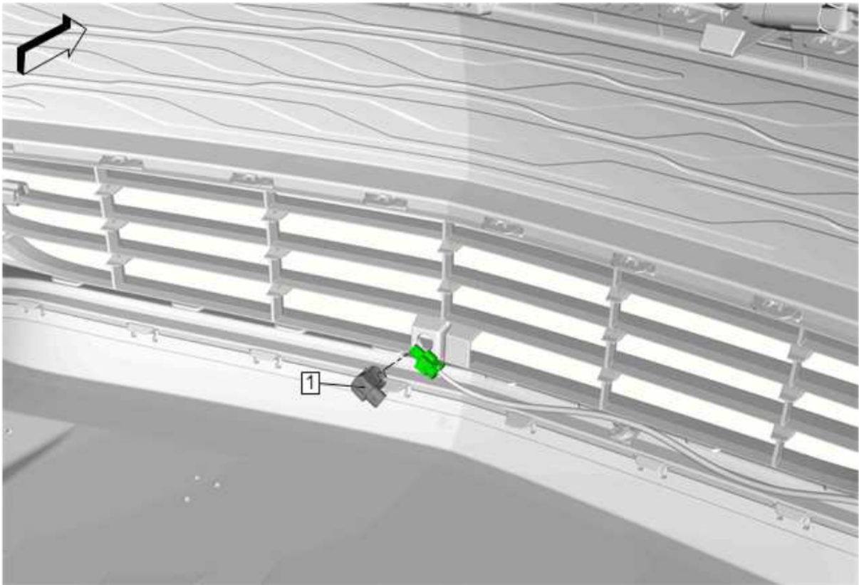
Fig. 5: Ambient Air Temperature Sensor Courtesy of GENERAL MOTORS COMPANY
