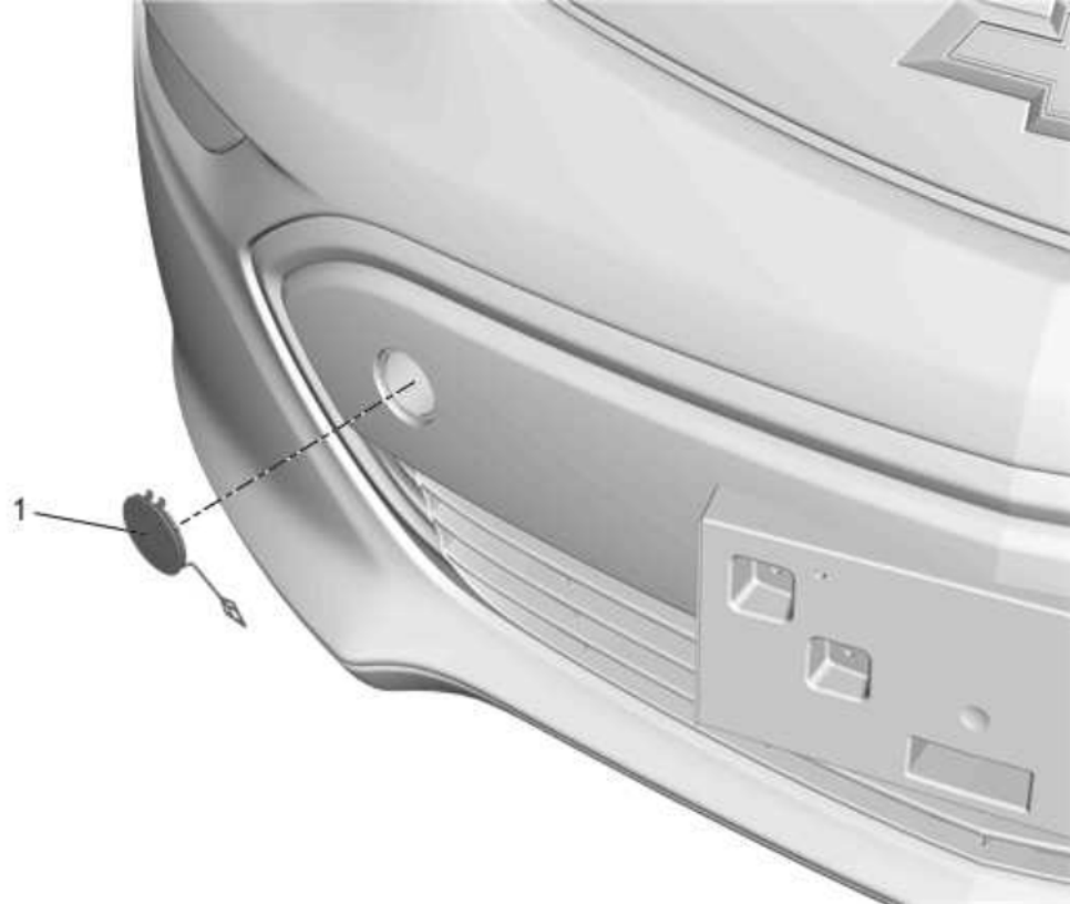
Fig. 12: Front Bumper Fascia Tow Eye Access Hole Cover Courtesy of GENERAL MOTORS COMPANY
