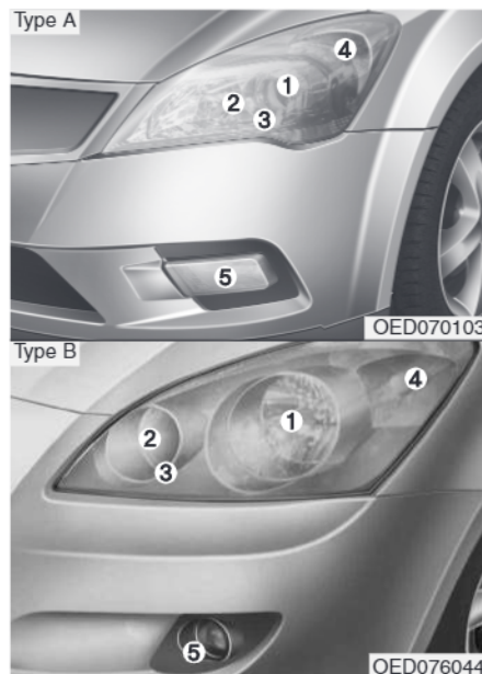
Headlight, position light, turn signal light, front fog light bulb replacement
