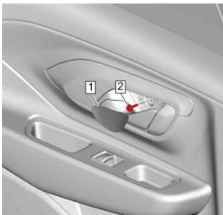
Fig. 92: Rear Side Door Inside Handle Fastener And Bolt Finish Cap Courtesy of GENERAL MOTORS COMPANY
