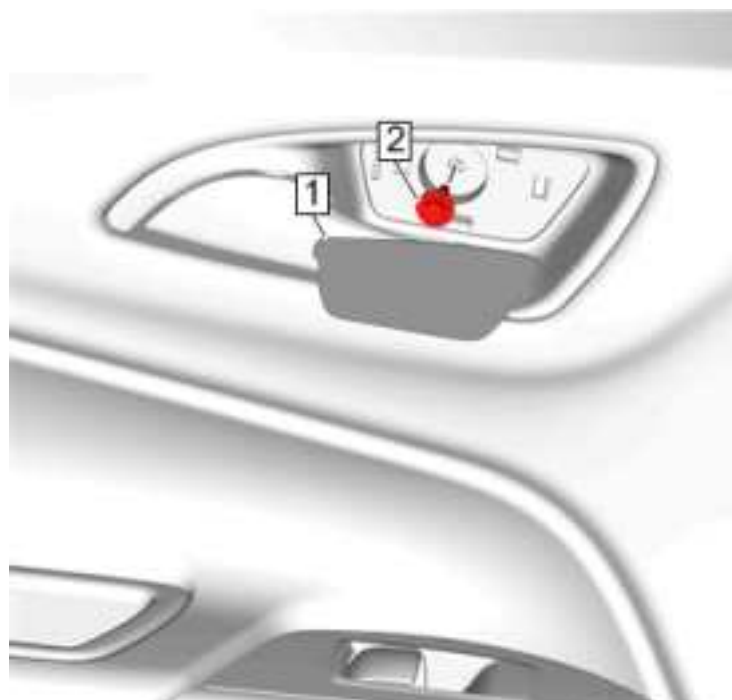
Fig. 79: Rear Side Door Inside Handle Fastener And Bolt Finish Cap Courtesy of GENERAL MOTORS COMPANY
