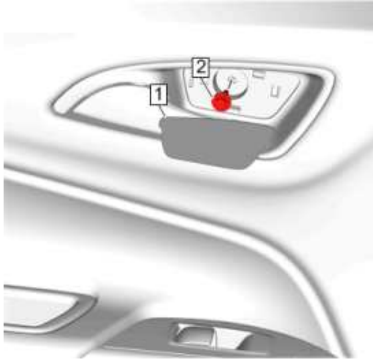
Fig. 85: Rear Side Door Inside Handle Fastener And Bolt Finish Cap Courtesy of GENERAL MOTORS COMPANY
