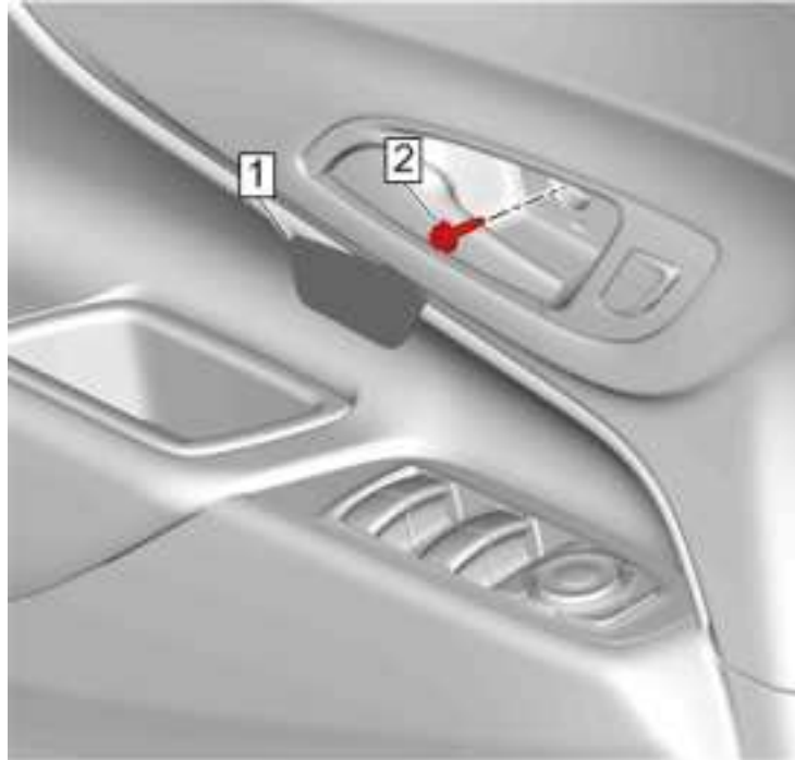
Fig. 9: Front Side Door Inside Handle Bolt Finish Cap
