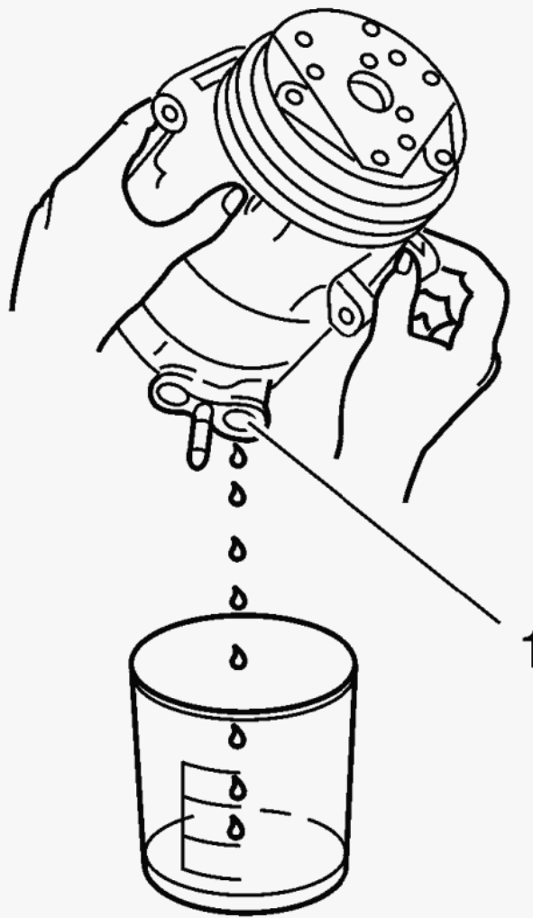
Fig. 9: Draining And Measuring Refrigerant Oil Courtesy of GENERAL MOTORS COMPANY
