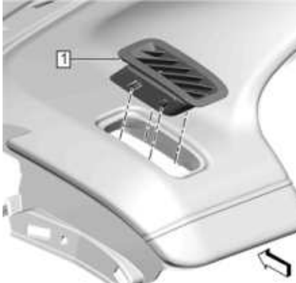
Fig. 936: Window Defogger Outlet Grille Courtesy of GENERAL MOTORS COMPANY
