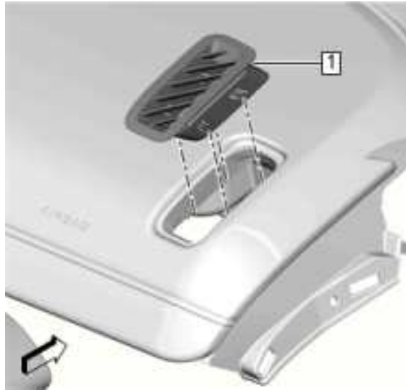
Fig. 934: Window Defogger Outlet Grille Courtesy of GENERAL MOTORS COMPANY
