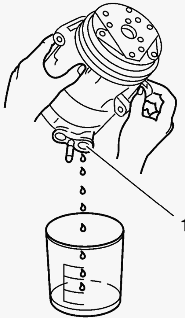
Fig. 10: Draining And Measuring Refrigerant Oil
