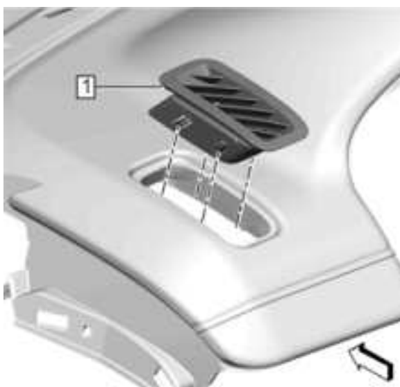
Fig. 933: Window Defogger Outlet Grille Courtesy of GENERAL MOTORS COMPANY
