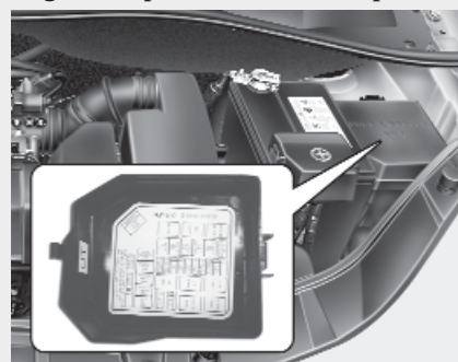
Engine compartment sub fuse panel (Diesel only)
