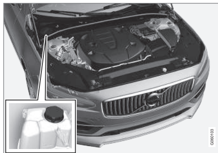
Coolant expansion tank
