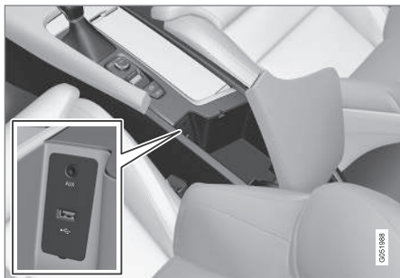
USB socket in the tunnel console
