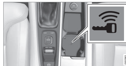
Back-up reader in the tunnel console
