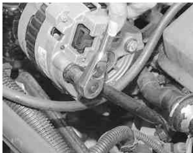
Fig. 6: Remove the alternator-to-brace bolt
