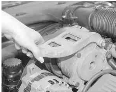
Fig. 5: . . . then swing the bracket up and away from the alternator
