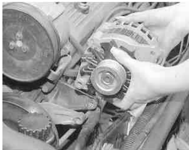
Fig. 9: . . . then remove the alternator from the vehicle
