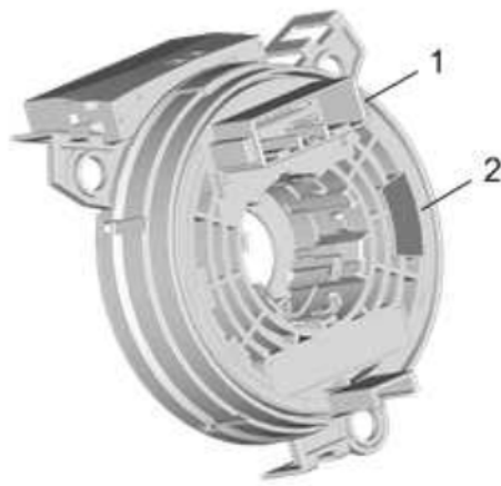
Fig. 33: Centering Steering Wheel Airbag Coil Courtesy of GENERAL MOTORS COMPANY
