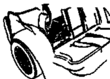
Fig. 111: Drive Motor Battery Cooling Blower Outlet Duct Fastener Courtesy of GENERAL MOTORS COMPANY
