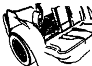
Fig. 104: Drive Motor Battery Cooling Blower Outlet Duct Fastener Courtesy of GENERAL MOTORS COMPANY
