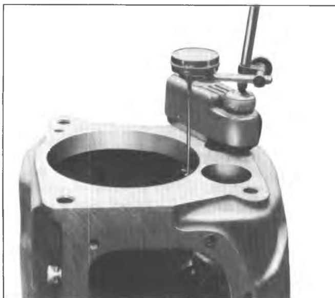
Fig. 7B-20K--Checking Countergear End Play
