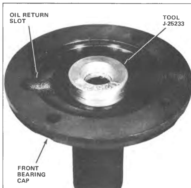
Fig. 7B-17B--Installing Clutch Bearing Retainer Seal
