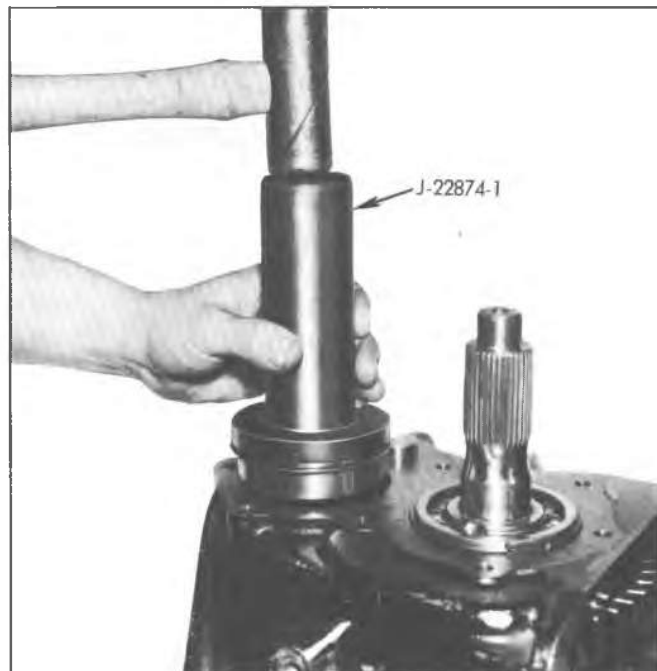
Fig. 7B-25L--Installing Countergear Rear Bearing
