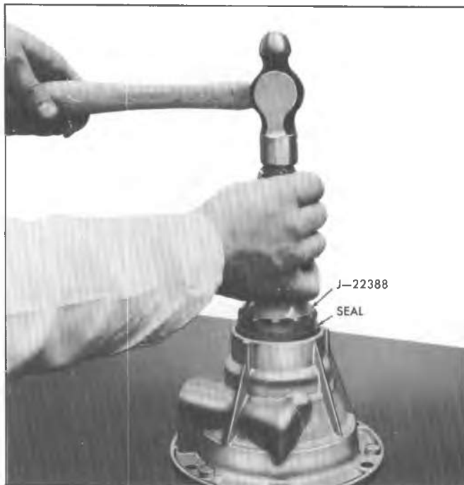
Fig. 7B-19S--Installing Rear Output Shaft Seal
