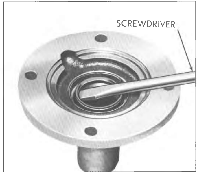
Fig. 7B-14J--Removing Bearing Retainer Oil Seal
