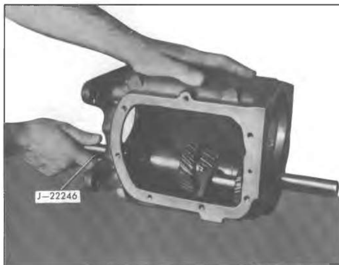
Fig. 7B-5A--Removing Counter Gear Shaft
