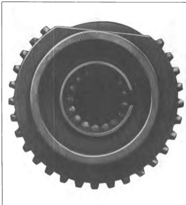
Fig. 7B-12L--Pilot Roller Bearing Installed
